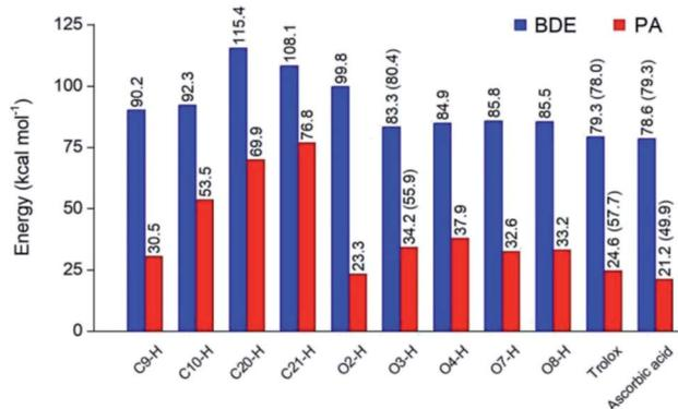
Fig. 2 Thermochemical properties including BDE and PA values (in kcal mol<sup>-1</sup>) for rosmarinic acid and trolox, ascorbic acid being used as the compounds of reference in water at 298.15 K calculated at the M05-2X/6-311++G(2df,2p) level of theory. The values in parentheses correspond to the results obtained in the PEA phase.
