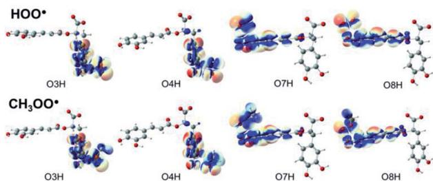
**Fig. 5** SOMO distributions of the transition states (TSs) for FHT reactions between RA<sup>-</sup> with HOO<sup>•</sup> and CH<sub>3</sub>OO<sup>•</sup> radicals in the aqueous phase.
