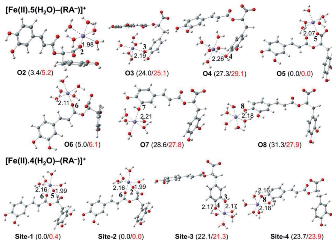
Fig. 6 Optimized structures of 7 monodentate complex types and 4 bidentate ones between the rosmarinic acid mono-anion ( $\text{RA}^-$ ) and the  $[\text{Fe(II)}(\text{H}_2\text{O})_6]^{2+}$  ion in water. The numbers in parentheses are the relative values for standard enthalpies (in black) and Gibbs free energies (in red) (in kcal mol<sup>-1</sup>) of  $\text{Fe(II)}$  complexes at 298.15 K.
