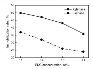
Effect curves of EDC concentration on enzyme immobilization Fig. 4 rate
