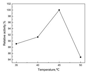
Fig. 6 Effect curve of temperature on degradation efficiency.
