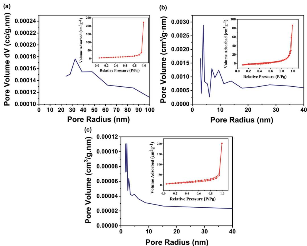
Fig. 6 The pore size distribution obtained for the designed membrane with different concentrations of FMWCNTs in fixed filtration volume. Insets show the corresponding  $N_2$  adsorption/desorption isotherms. (a) 0.3 g, (b) 0.4 g, and (c) 0.5 g, showing that the pore size of the designed FMWCNTs membrane has been tuned from 27.4 nm to 1.7 nm by choosing different concentrations of FMWCNTs.
