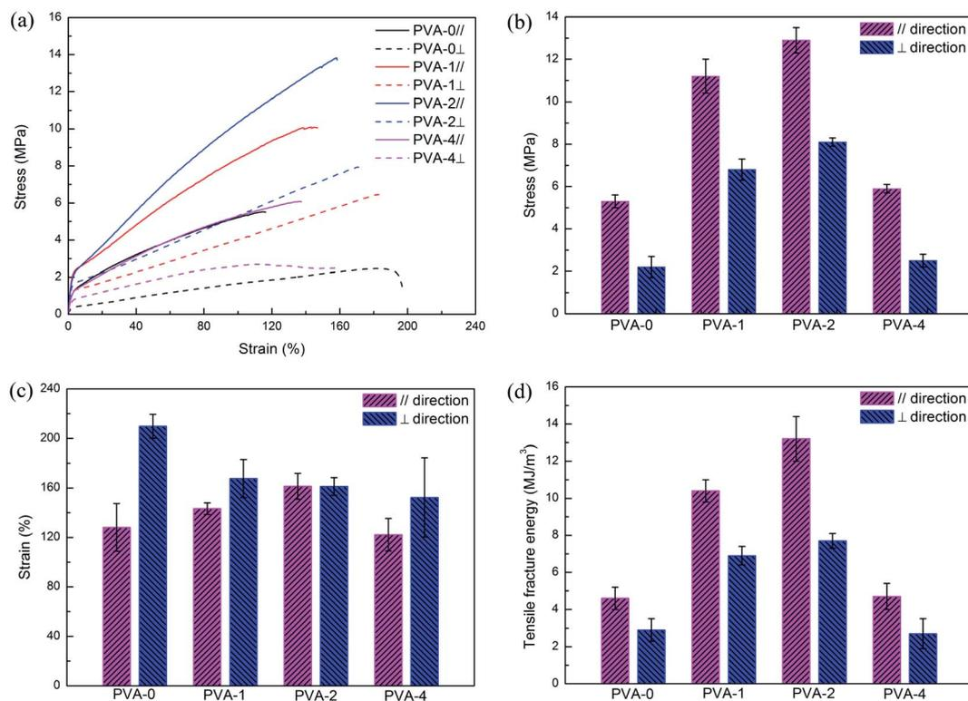
Fig. 5 Mechanical properties of the interpenetrating network PVA/alginate hydrogels with different mass fractions of PVA along (||) and perpendicular ( $\perp$ ) to the fibrous directions: tensile stress–strain curves (a), tensile stress (b), tensile strain (c) and tensile fracture energy (d).
