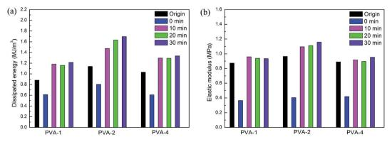
Fig. 7 Dissipated energy (a) and elastic modulus (b) of a single loading-unloading test at a strain of 30% after different resting times for the interpenetrating network PVA/alginate hydrogel with hierarchical fibrous structures.
