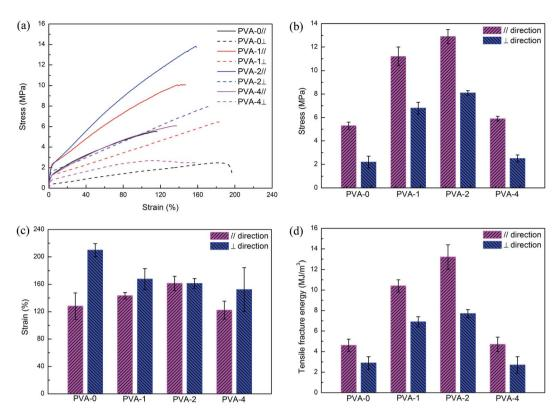
Fig. 5 Mechanical properties of the interpenetrating network PVA/alginate hydrogels with different mass fractions of PVA along (||) and perpendicular (\(\pm\)) to the fibrous directions: tensile stress-strain curves (a), tensile stress (b), tensile strain (c) and tensile fracture energy (d).
