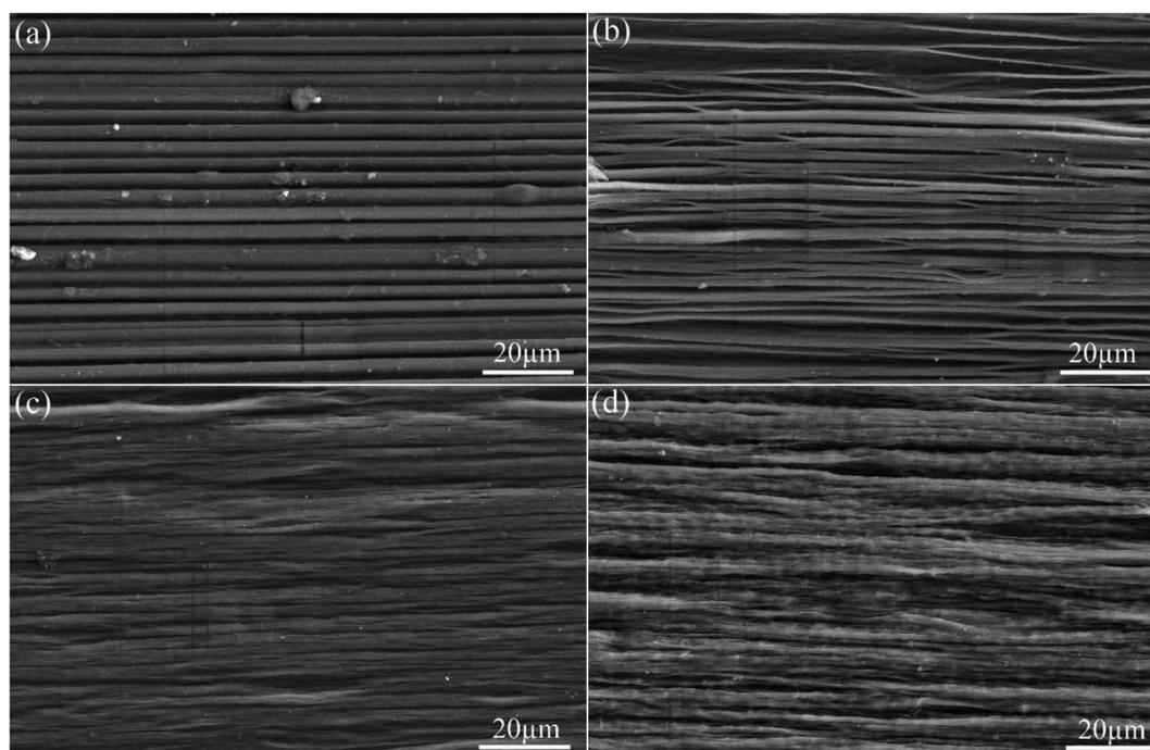
Fig. 3 Typical SEM images of the interpenetrating network PVA/alginate hydrogel with hierarchical fibrous structures containing 0 wt% (a) 1 wt% (b), 2 wt% (c), 4 wt% (d) of PVA.
