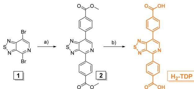
Scheme 2 Synthetic route for H<sub>2</sub>-TDP. Reagents and conditions: (a) Cs<sub>2</sub>CO<sub>3</sub>, CsF, Pd(PPh<sub>3</sub>)<sub>4</sub>, Pd(dppf)Cl<sub>2</sub>, toluene–H<sub>2</sub>O, 90 °C for 2 d; (b) KOH, THF, CH<sub>3</sub>OH, H<sub>2</sub>O, 90 °C for 2 h; TFA, H<sub>2</sub>O, 0.5 h, room temperature.
