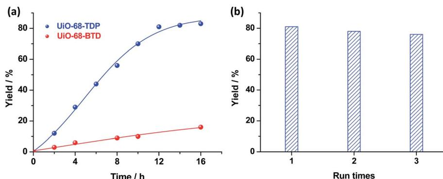
Fig. 2 (a) Photocatalytic profiles of oxidative annulation reaction between *N,N*-dimethylaniline (1a) and *N*-(4-methylphenyl)maleimide (2a) by UiO-68-TDP and UiO-68-BTD under the irradiation of blue-LEDs in an open air atmosphere. (b) Recycling experiments of UiO-68-TDP for the photocatalyzed oxidative annulation reaction.
