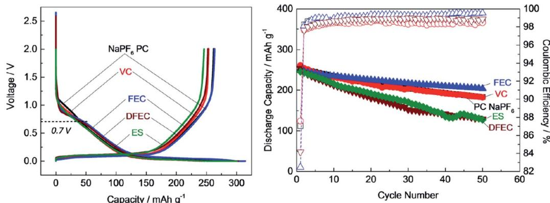
Fig. 3 Cycle performance of hard-carbon anode in 1 mol dm<sup>-3</sup> NaPF<sub>6</sub> in PC-based electrolyte containing 1 vol% of FEC, VC, ES and DFEC additives.<sup>23</sup> Copyright 2016, John Wiley & Sons, Inc.
