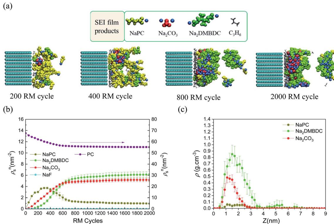
Fig. 2 (a) Typical snapshots of SEI layer formation during RM cycles in PC-based electrolyte solution. (b) Surface number densities ( $\rho_s^n$ ) of SEI film products and solvent molecules,<sup>60</sup> and (c) mass density distributions ( $\rho$ ) of SEI products.<sup>60</sup> Copyright 2018, American Chemical Society.
