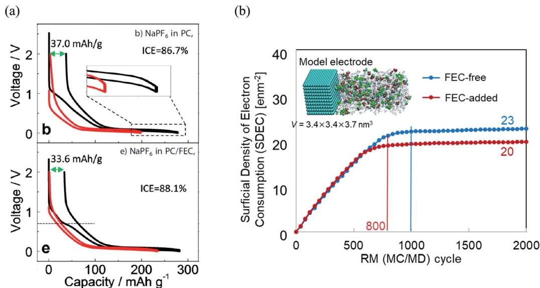
Fig. 5 (a) Charge/discharge curves (1<sup>st</sup> cycle, black line; 30<sup>th</sup> cycle, red line) of carbon-based electrode cycled<sup>23</sup> (Copyright 2016, John Wiley & Sons, Inc.), and (b) the electron consumption used for SEI film formation in NaPF<sub>6</sub> PC/FEC based electrolyte on carbon-based electrode.
