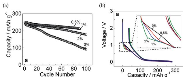
Fig. 7 (a) Capacity retention and (b) initial charge/discharge of hard-carbon electrodes cycled in 1 mol dm<sup>-3</sup> NaPF<sub>6</sub> PC-based electrolyte containing 0, 0.5, 1, and 2 vol% of FEC concentration.<sup>23</sup> Copyright 2016, John Wiley & Sons, Inc.
