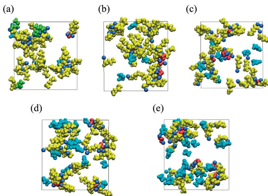
Fig. 9 Typical snapshot of SEI film at initial stage of formation (red,  $\text{Na}_2\text{CO}_3$ ; green,  $\text{Na}_2\text{DMBDC}$ ; dark yellow, NaPC; pink, NaF; cyan blue, FEC) in  $\text{NaPF}_6/\text{PC}$  electrolyte solution containing (a) 1, (b) 3, (c) 5, (d) 7 and (e) 10 vol% of FEC additive concentration.<sup>60</sup> Copyright 2018, American Chemical Society.
