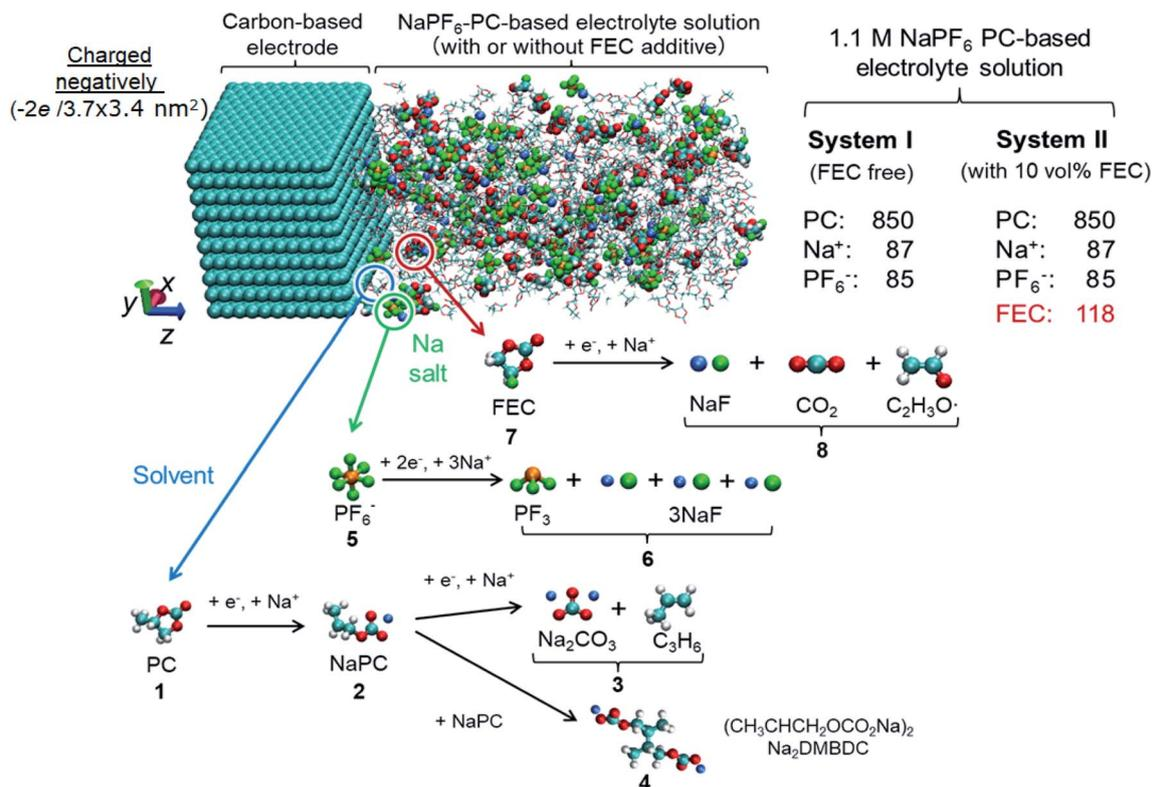
Fig. 1 Model simulation system and reaction schemes in the PC-based electrolyte. (cyan: C, red: O, white: H, orange: P, green: F, blue: Na<sup>+</sup>).
