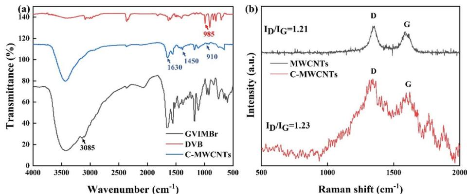
Fig. 3 (a) FTIR spectra of GVIMBr, DVB and C-MWCNTs, and (b) Raman images of MWCNTs and C-MWCNTs.
