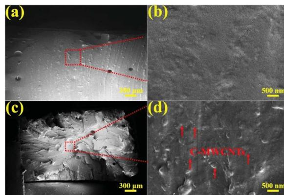
Fig. 10 (a and c) SEM images of (a) neat PUE and (c) C-MWCNTs/PUE fracture, and (b and d) High magnification SEM images corresponding to the selected area in (a and c).
