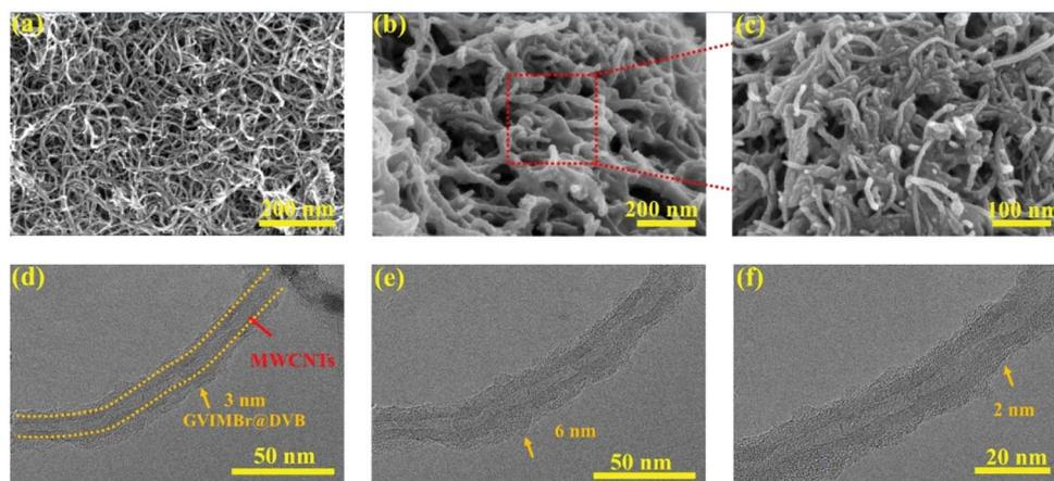
Fig. 5 (a) SEM images of MWCNTs, (b) SEM images of GVIMBr and DVB coated MWCNTs, (c) SEM images of GVIMBr and DVB coated MWCNTs corresponding to the selected area in (b), and (d)–(f) TEM images of C-MWCNTs with coating structure.
