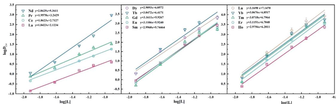
**Fig. 4** Dependency of  $\log D_{Ln}$  on extractant concentration in 40/60 (v/v)% *n*-octanol/kerosene (O : A = 1 : 1),  $[\text{Ln}^{3+}]_{\text{init}} = 3 \text{ mM}$ ,  $[\text{L}^{\text{II}}] = 0.012\text{--}0.12 \text{ M}$ .
