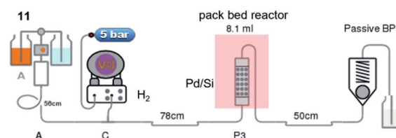
Fig. 1 Hydrogenation of diethyl oximinomalonate ( 11 ) in a continuous flow reactor.
