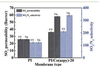
Fig. 11 The light-responsive characteristic of the Co(azpy)-loaded MMM for  $SO_2/N_2$  separation performance.
