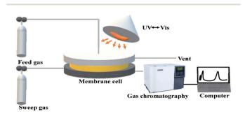
**Scheme 3** The diagrammatic sketch of the gas membrane separation apparatus.
