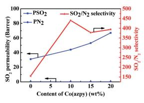
Fig. 10 The influence of the Co(azpy) content on the  ${\rm SO_2/N_2}$  separation performance.
