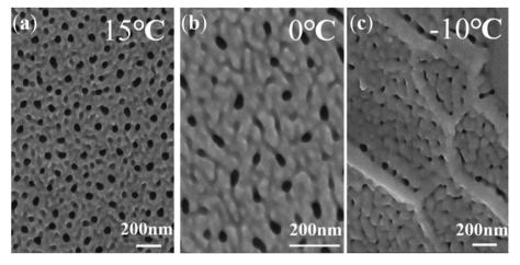
Fig. 3 FESEM images showing the surface morphologies of nanotubes anodized at a constant voltage (60 V) for 600 s at different temperatures: (a) 15  $^{\circ}$ C, (b) 0  $^{\circ}$ C, (c) -10  $^{\circ}$ C.
