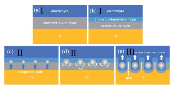
Fig. 2 Diagram of the 'oxygen bubble model' growth.
