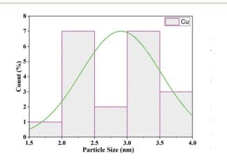
Fig. 9 Particle size distribution of Cu/zeolite-Y.
