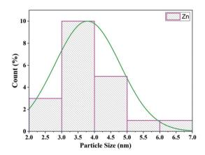
Fig. 11 Particle size distribution of Zn/zeolite-Y.
