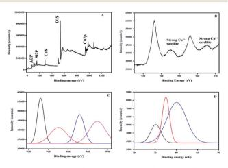
Fig. 7 XPS spectra of Cu/zeolite-Y: (A) survey, (B) Cu 2p, (C) Gaussian curves for Cu 2p, and (D) Gaussian curves for Al 2p.
