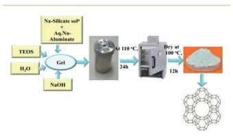
Scheme 1 Preparation of zeolite-Y.
