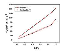
Fig. 14  $\,$  N $_2$  adsorption—desorption isotherms of zeolite-Y and Cu/zeolite-Y catalysts.
