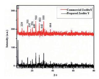
Fig. 3 X-ray diffraction patterns of commercial and prepared zeolites-v
