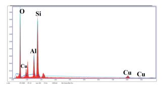
Fig. 6 EDS elemental analysis of Cu/zeolite-Y.
