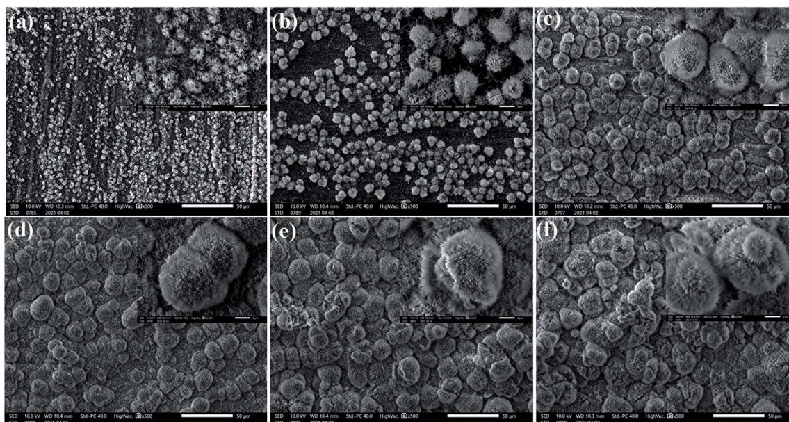
Fig. 1 SEM images of the cathodic copper surface in 0.1 M myristic acid and 0.2 M calcium chloride solution with a DC voltage of 30 V for different electro-deposition times: (a) 0.5 min; (b) 1 min 35 s; (c) 10 min; (d) 15 min; (e) 30 min; (f) 45 min.
