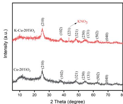
Fig. 2 XRD patterns of Cu-20TiO<sub>2</sub> and K-Cu-20TiO<sub>2</sub>.
