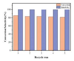
Fig. 6 Recycling of the catalyst.
