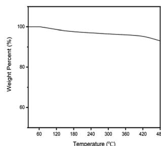
Fig. 3 TG curve of K-Cu-20TiO<sub>2</sub>.
