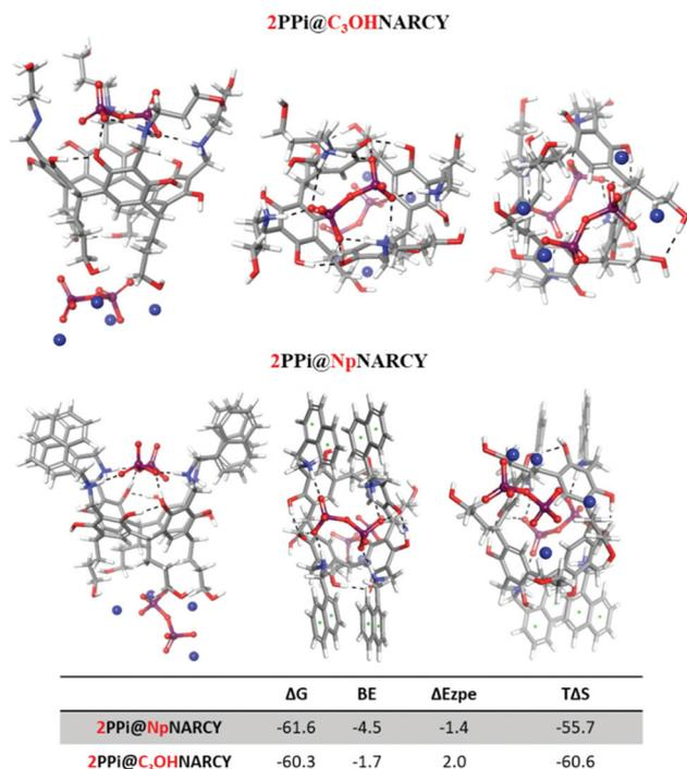
**Fig. 8** The optimized geometry of 2PPI@NpNAR and 2PPI@C<sub>3</sub>OHNAR complexes. Side view, top-down view, bottom-up view. BE is binding energy,  $E_{zpe}$  is the zero-point energy; these terms together equate to  $\Delta H$ .
