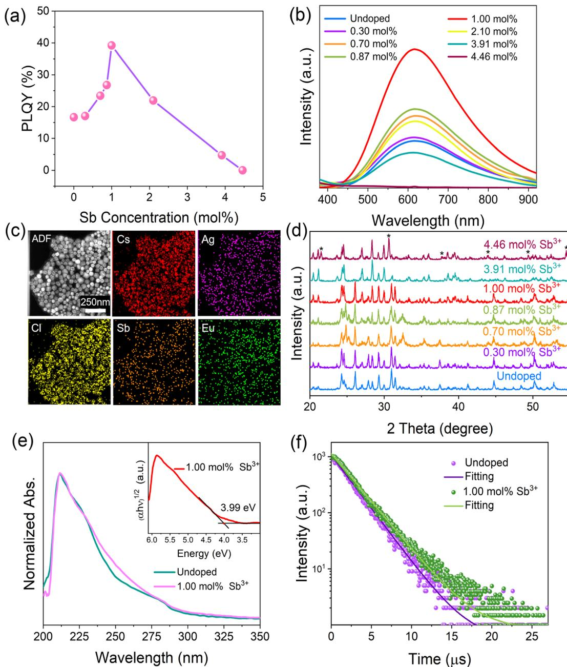
**Fig. 2** (a) PLQY and (b) PL spectra of CsAgCl<sub>2</sub> NCs with different Sb<sup>3+</sup> doping levels. (c) TEM-EDS elemental mapping results of 1.0 mol% Sb-doped NCs. (d) XRD patterns of 0–4.46 mol% Sb-doped NCs. (e) UV-vis absorption spectra (the inset shows the Tauc plot for the doped NCs) and (f) TRPL curves measured for the undoped and 1.0 mol% Sb-doped NCs at 300 K, monitoring the same emission peak at 625 nm.
