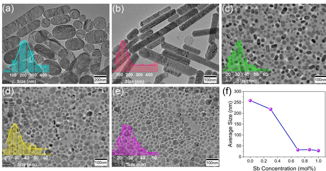
Fig. 4 TEM images of CsAgCl<sub>2</sub> NCs prepared with different Sb<sup>3+</sup> doping levels. (a) 0 mol%, (b) 0.3 mol%, (c) 0.70 mol%, (d) 0.87 mol%, and (e) 1.00 mol%. (f) Particle size of the CsAgCl<sub>2</sub> NCs as a function of Sb<sup>3+</sup> doping concentration.
