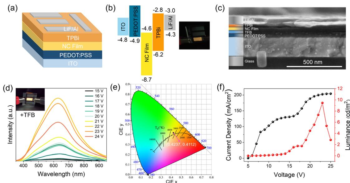
Fig. 5 (a) Device structure and (b) energy band diagram (relative to the vacuum level) of the Sb-doped CsAgCl<sub>2</sub> NC LEDs. Inset: photograph of an LED driven by a 14 V bias. (c) Cross-sectional SEM image of a TFB-incorporated device. (d) EL spectra of the resulting LEDs at different applied voltages. Inset: photograph of the LED driven by a 22 V bias. (e) CIE coordinates and (f) *I*–*V*–*L* characteristics of the LED devices.
