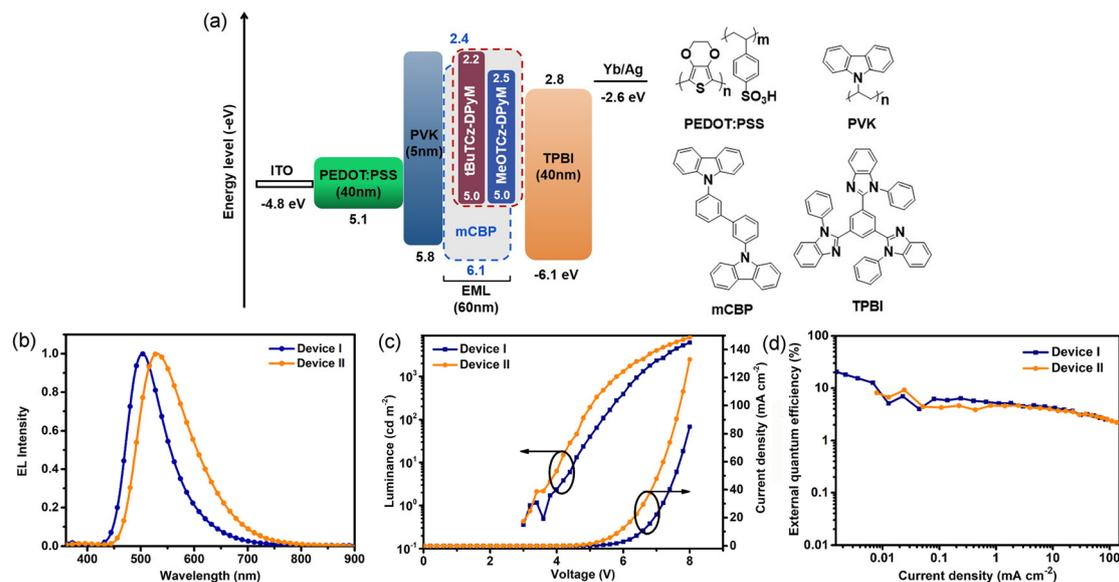
Fig. 4 (a) Relative energy-level alignment of the devices (left) and chemical structures of the materials (right); (b) EL spectra of the devices; (c) current density–voltage–luminance ( $J$ – $V$ – $L$ ) characteristics of the devices; and (d) external quantum efficiency–current density characteristics of the devices.
