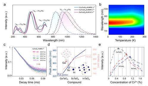
Fig. 2 (a) PLE and PL spectrum of  $XTaO_4$ :  $Cr^{3+}$  (X = In, Sc, and Ga); (b) the low-temperature emission spectra of  $GaTaO_4$ :  $Cr^{3+}$ ; (c) decay curves of GaTaO<sub>4</sub>:Cr<sup>3+</sup> were monitored at 810 nm, 860 nm, 910 nm, 960 nm, and 1010 nm; (d) variation trend of the PL intensity of XTaO<sub>4</sub>:Cr<sup>3+</sup>(X = In, Sc, and Ga) with  $Cr^{3+}$ -ion concentration; (e) the peaking position and FWHM of XTaO<sub>4</sub>: $Cr^{3+}$  (X = In, Sc, and Ga).
