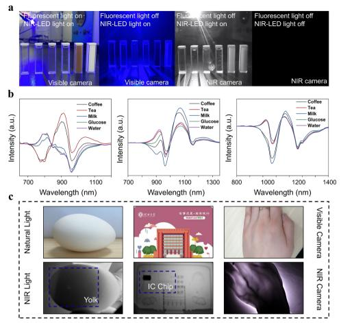
Fig. 5 A multitude of applications of XTaO<sub>4</sub>:Cr<sup>3+</sup> (X = In, Sc, and Ga) are demonstrated; (a) night vision (visual and NIR images of water, glucose, tea, milk, and coffee); (b) nondestructive food detection (NIR spectra after penetrating water, glucose, tea, milk, and coffee); (c) NIR non-destructive testing applications (photos of eggs, access cards and palms in natural and NIR light).
