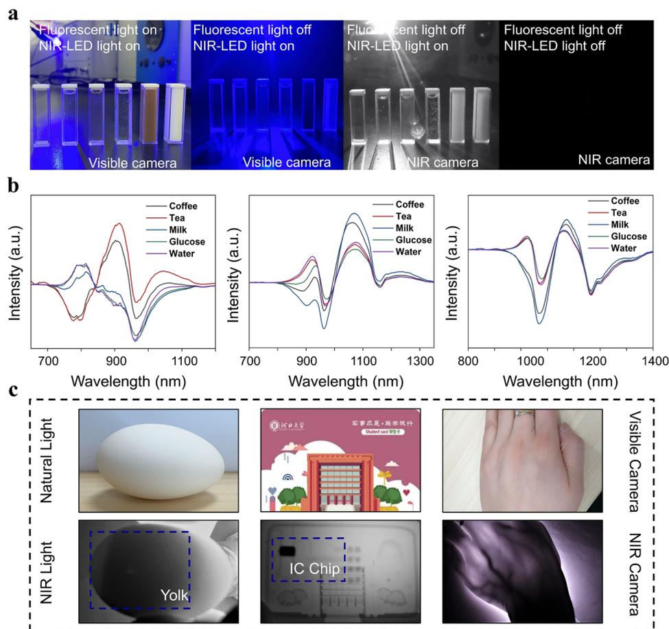
Fig. 5 A multitude of applications of  $\text{XTaO}_4:\text{Cr}^{3+}$  ( $X = \text{In}, \text{Sc}, \text{and Ga}$ ) are demonstrated; (a) night vision (visual and NIR images of water, glucose, tea, milk, and coffee); (b) nondestructive food detection (NIR spectra after penetrating water, glucose, tea, milk, and coffee); (c) NIR non-destructive testing applications (photos of eggs, access cards and palms in natural and NIR light).
