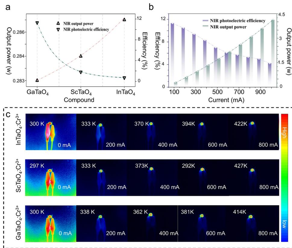
Fig. 4 (a) Output optical powers, and conversion efficiencies of the NIR-LED of  $XTaO_4:Cr^{3+}$  ( $X = In, Sc, and Ga$ ) depending on the 100 mA driving current; (b) output optical powers, and conversion efficiencies of the NIR-LED of  $GaTaO_4:Cr^{3+}$  depending on the driving current from 100 mA to 1000 mA; (c) thermal images of the pc-LED of  $XTaO_4:Cr^{3+}$  ( $X = In, Sc, and Ga$ ) at different operating currents over 0–800 mA.
