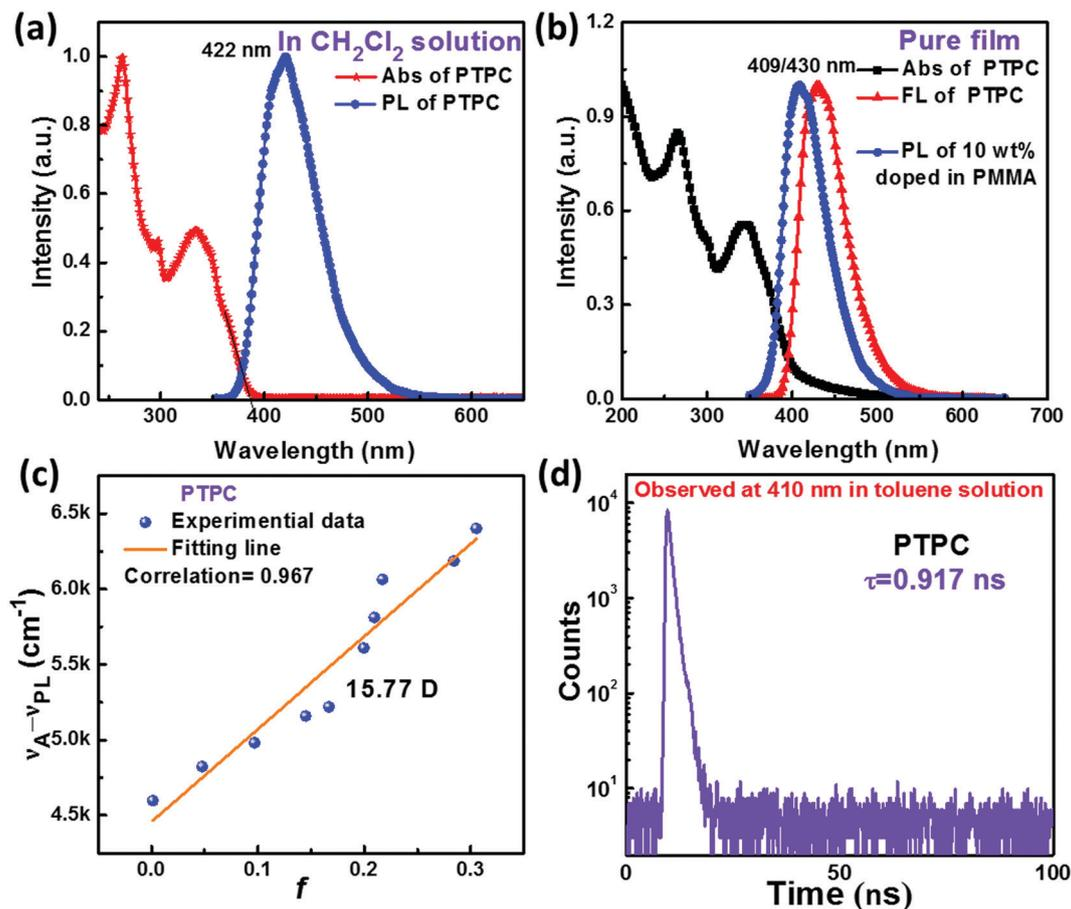
Fig. 3 (a) UV-Vis absorption and PL spectra of PTPC in  $\text{CH}_2\text{Cl}_2$  solution (10  $\mu\text{M}$ ). (b) UV-Vis absorption and PL spectra of PTPC in neat films and the PL spectrum of 10 wt% PTPC doped into PMMA. (c) Solvatochromic Lippert–Mataga models of PTPC with the Stokes shift ( $\nu_a - \nu_f$ ) versus orientational polarizability ( $f$ ). (d) Transient PL decay curve in toluene solution at an excitation of 280 nm.
