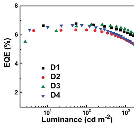
Fig. 5 EQE versus luminance curves of the deep-blue devices (**D1**, **D2**, **D3** and **D4**).
