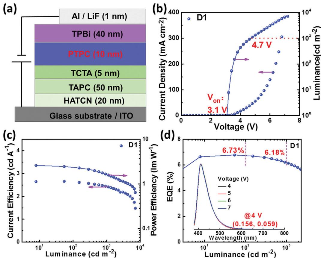
Fig. 4 The device structure diagram and EL performance of **D1**. (a) Device structure diagram. (b) Current density and luminance versus voltage curves. (c) Current efficiency and power efficiency versus luminance curves. (d) EQE versus luminance curves. The inset shows the normalized EL spectra at different voltages.
