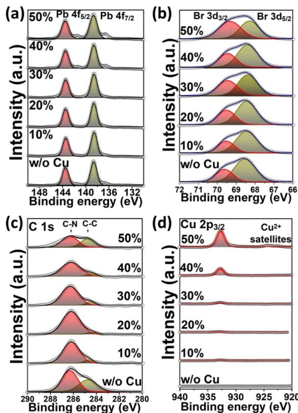
Fig. 4 XPS spectra of Pb4f (a), Br3d (b), C1s (c), and Cu2p (d), and Br3d (e) of Cu-alloyed MAPbBr<sub>3</sub> perovskite thin films.
