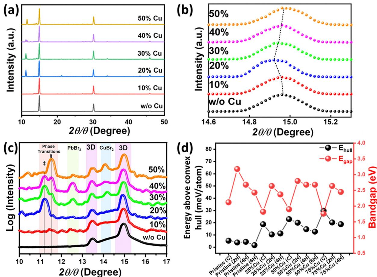
Fig. 3 (a) XRD patterns of Cu-alloyed MAPbBr<sub>3</sub> perovskite thin films. (b) XRD peak (100) shift upon copper addition. (c) XRD patterns (log scale) for  $2\theta = 10\text{--}17^\circ$ . (d) Energy above convex hull and bandgap for different phases of pure and Cu-alloyed MAPbBr<sub>3</sub> where C, 2H, 4H, and 6H represent cubic, hexagonal-2H, hexagonal-4H, and hexagonal-6H phases of MAPbBr<sub>3</sub>, respectively.
