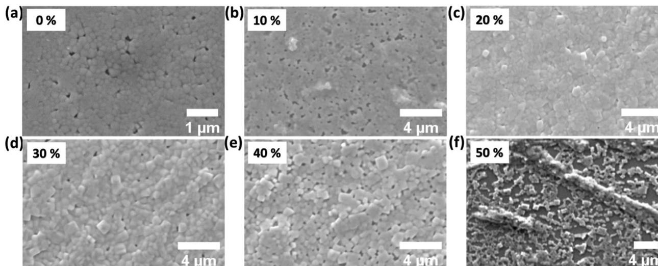
Fig. 2 SEM images of undoped (a), 10% (b), 20% (c), 30% (d), 40% (e), and 50% (f) Cu-alloyed MAPbBr<sub>3</sub> thin films.
