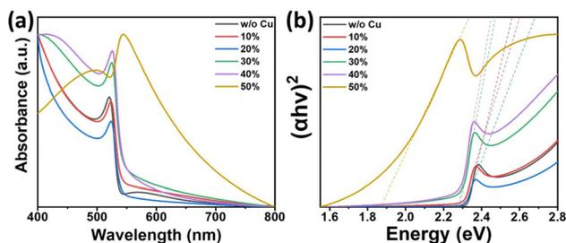
Fig. 5 (a and b) Absorption spectra, and direct bandgap estimation: Tauc plot, respectively, of Cu-alloyed MAPbBr<sub>3</sub> thin films.
