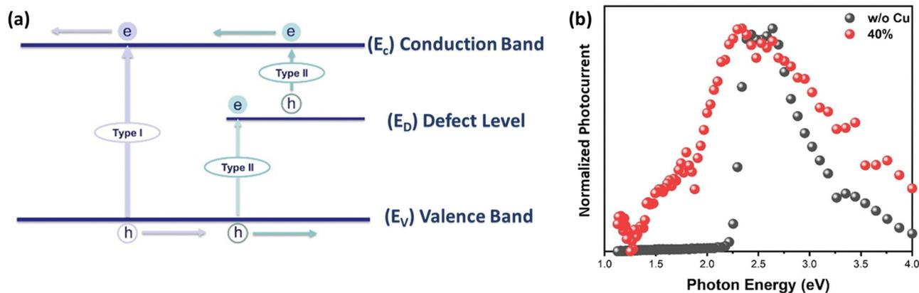
Fig. 7 (a) Graphical illustration of photo-excitation processes in Cu-alloyed MAPbBr<sub>3</sub> perovskite and (b) Photocurrent spectra of pristine MAPbBr<sub>3</sub> and 40% Cu-alloyed MAPbBr<sub>3</sub> thin films at room temperature.
