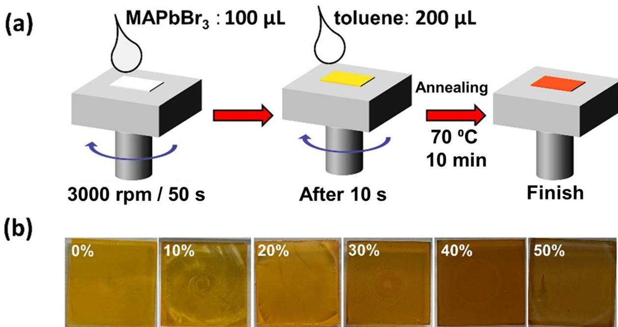
**Fig. 1** (a) Graphical illustration of perovskite thin film fabrication *via* spin-coating. (b) Picture of pristine (0%) and (10, 20, 30, 40, and 50%) Cu-substituted MAPbBr<sub>3</sub> thin films obtained from use of (0, 10, 20, 30, 40, and 50%) [CuBr<sub>2</sub>]/([CuBr<sub>2</sub>] + [PbBr<sub>2</sub>]) mole percentages.
