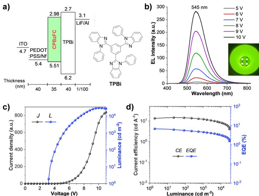
**Fig. 5** (a) Device structure and energy levels (relative to the vacuum energy level) and the molecular structure of the organic material used. (b) EL spectra at various applied voltages (inset: photograph of the glowing OLED device). (c) Current density–voltage–luminance ( $J$ – $V$ – $L$ ) characteristics and (d) current efficiency–current density–EQE ( $CE$ – $J$ – $EQE$ ) plots.
