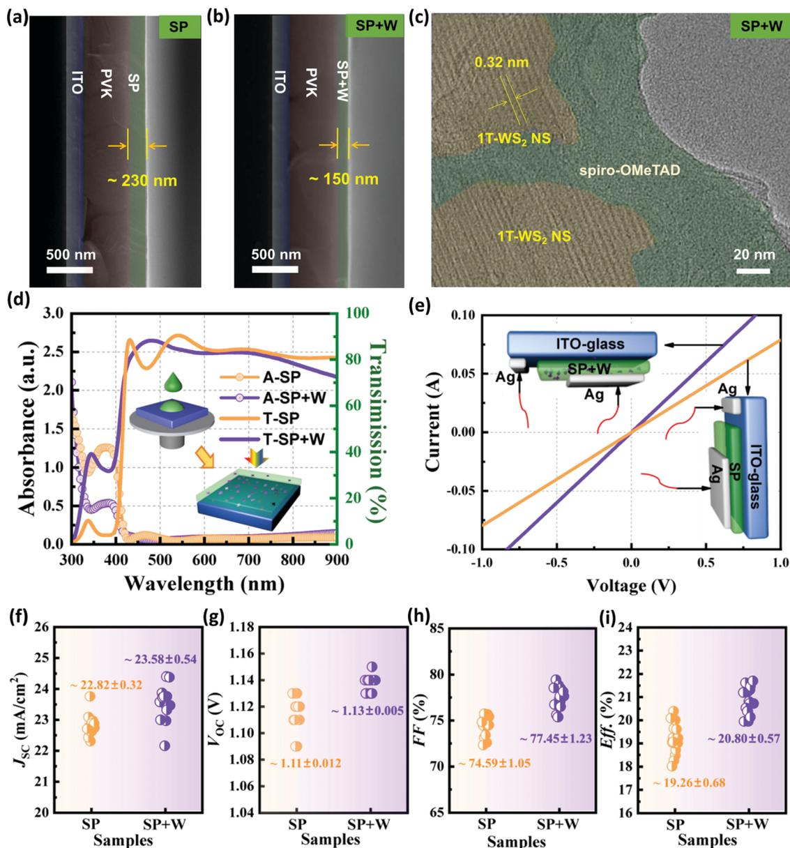
Fig. 2 Cross-sectional SEM images of (a) ITO/PVK/SP and (b) ITO/PVK/SP + W samples. (c) HRTEM image of the SP + W hybrid HTL. (d) Optical properties of ITO/SP and ITO/SP + W substrates. (e)  $J$ - $V$  characteristics of corresponding samples. Statistical analysis of the (f)  $J_{sc}$ , (g)  $V_{oc}$ , (h) FF, and (i) efficiency of 30 individual devices with different HTLs prepared under the same conditions.
