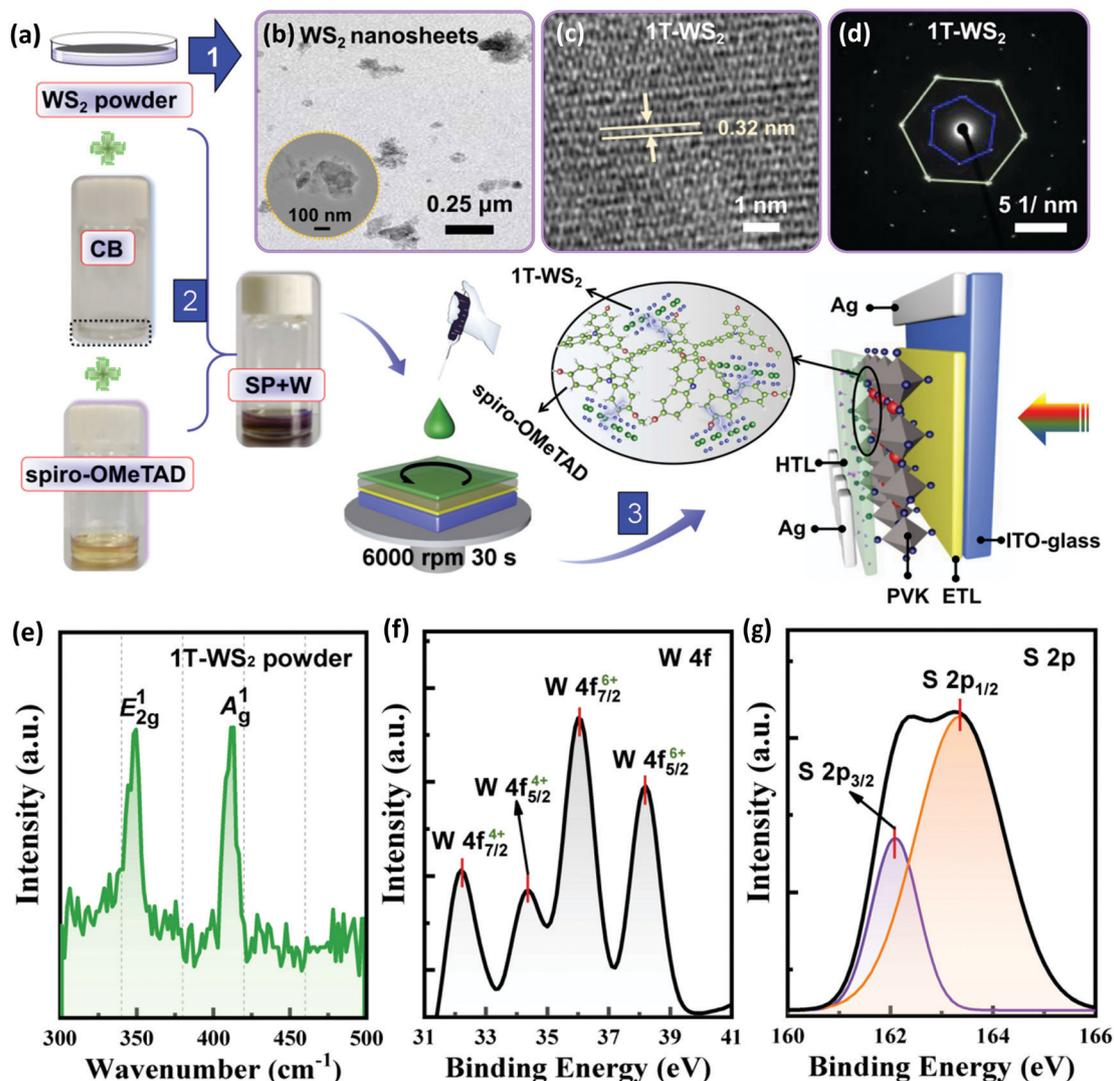
**Fig. 1** (a) Schematic of the manufacturing process of the SP + W hybrid HTL. Micrographs of commercial WS<sub>2</sub> nanosheets: (b) TEM image, (c) HRTEM image, and (d) SAED pattern. (e) Raman spectrum of the WS<sub>2</sub> nanosheets coated on the SiO<sub>2</sub> substrate. Corresponding high-resolution XPS profiles: (f) W 4f and (g) S 2p.
