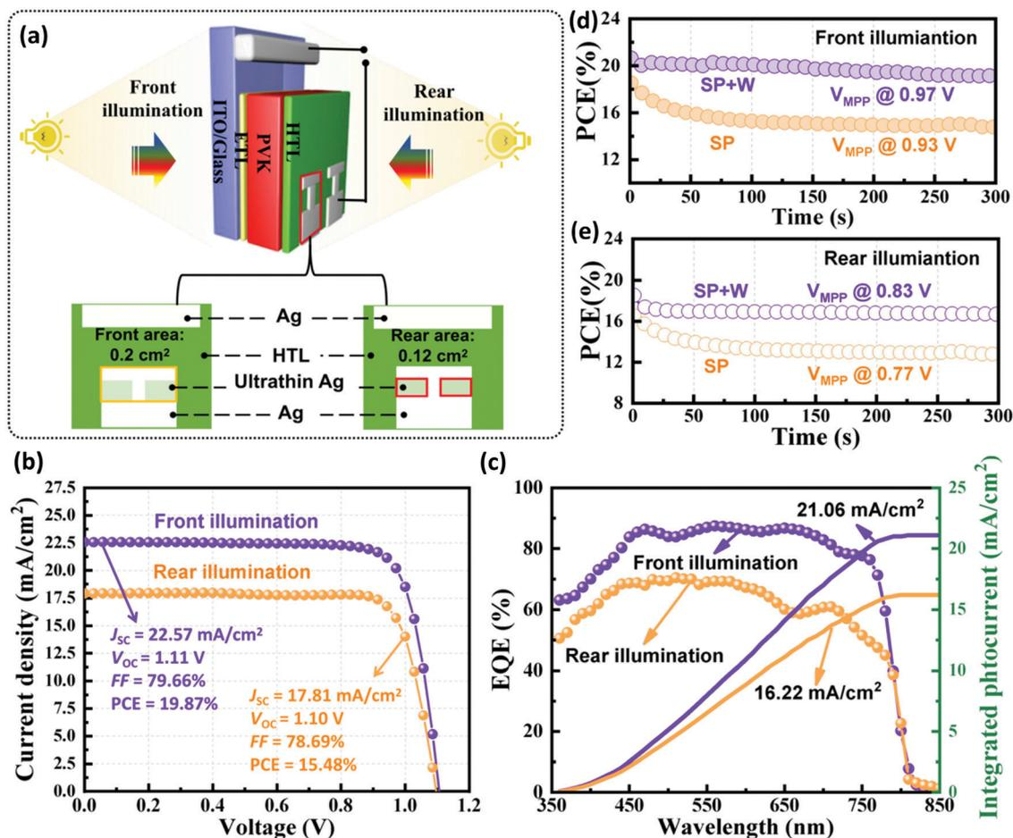
Fig. 4 (a) Structure and PV test model of the b-PSC. (b)  $J$ - $V$  characteristics and (c) corresponding EQE spectra of the best-performing SP + W b-PSC illuminated on different sides. (d) and (e) Steady-state PCEs measured at the voltage of the maximum power point for the two b-PSCs.
