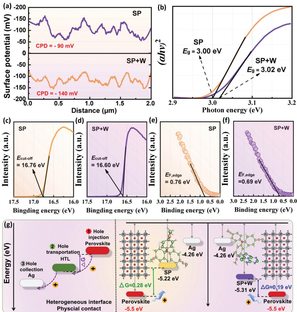
Fig. 3 (a) KPFM images and (b) Tauc plots of SP and SP + W samples. (c and d) UPS cut-off edge ( $E_{\text{cut-off}}$ ) and (e and f) Fermi edge ( $E_{\text{F,edge}}$ ) of the corresponding samples. (g) Schematic illustration of the carrier injection/transfer/collection processes based on the two abovementioned HTLs, according to band-gap alignments.
