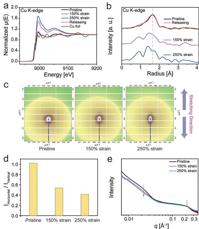
**Fig. 4** (a) XANES spectra of PU-SO-Cu under different strains. (b) EXAFS spectra of PU-SO-Cu under different strains. (c) 2D SAXS images of PU-SO-Cu with different extension strains during the uniaxial stretching process. (d) Ratio of intensities integrated in different directions (horizontal and vertical) under different strains. All intensities were calculated at  $q = 0.024 \text{ \AA}^{-1}$ . (e) 1D scattering profiles of PU-SO-Cu integrated from 2D SAXS patterns under different strains.
