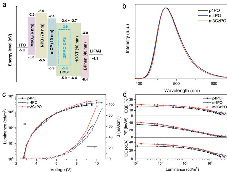
Fig. 5 (a) Energy level diagram of the OLEDs; (b) electroluminescence (EL) spectrum; (c) current density–luminance–voltage ( $J$ – $V$ – $L$ ) characteristics; and (d) external quantum efficiency (EQE), power efficiency (PE) and current efficiency (CE) versus luminance characteristics.
