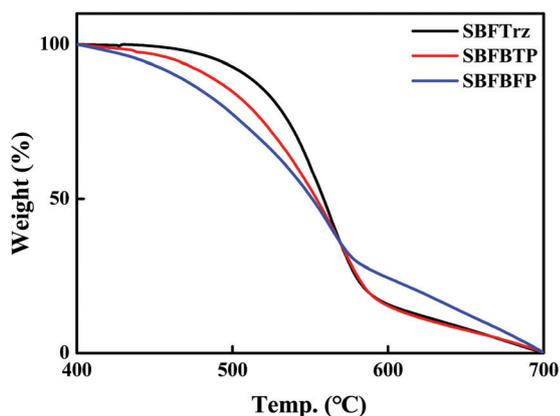
Fig. 2 TGA curves of SBFTTrz, SBFBTP and SBFBFP.
