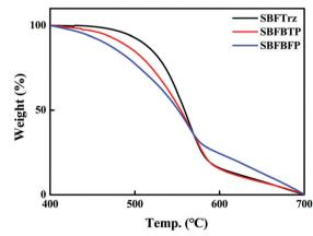
Fig. 2 TGA curves of SBFTrz, SBFBTP and SBFBFP.
