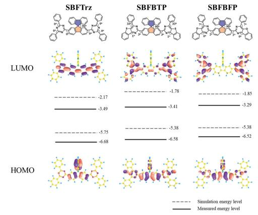
Fig. 1 Optimized geometry and HOMO and LUMO distribution and energy levels of SBFTrz, SBFBTP and SBFBFP.
