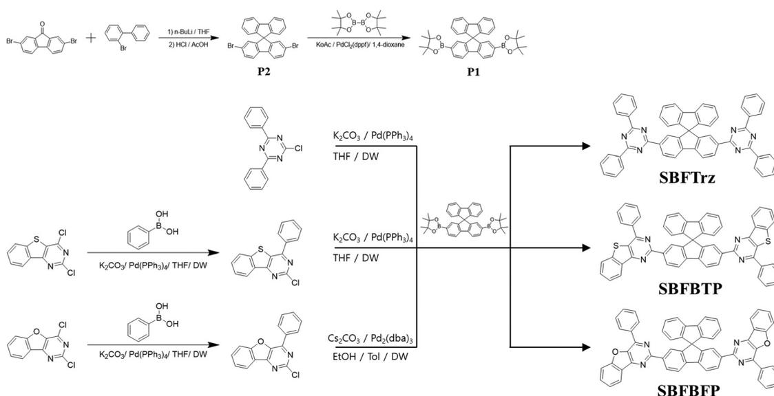
Scheme 1 Synthesis process of SBFTrz, SBFBTP and SBFBFP.
