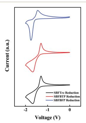
Fig. 4 Cyclic voltammetry (CV) curve of SBFTrz, SBFBTP and SBFBFP.
