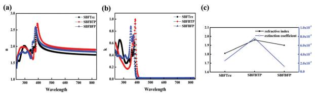
Fig. 9 (a) Refractive index and (b) extinction coefficient of the ETLs measured by spectroscopic ellipsometer, and (c) comparison of the refractive index and extinction coefficient of SBFTrz, SBFBTP and SBFBFP.
