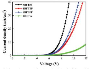
Fig. 5 Single carrier current densities of SBFTrz, SBFBTP and SBFBFP electron only devices.
