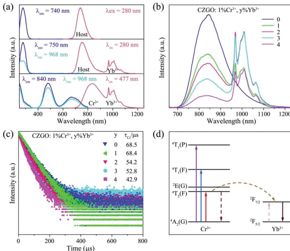
Fig. 6 (a) The PL and PLE spectra of the blank, and  $\text{Yb}^{3+}$ -doped and  $\text{Cr}^{3+}/\text{Yb}^{3+}$ -co-doped CZGO; (b) PL spectra and (c) decay curves of CZGO: 1%  $\text{Cr}^{3+}$ ,  $y\%$   $\text{Yb}^{3+}$  ( $y = 0, 1, 2, 3, 4$ ) excited by 480 nm light together with (d) an energy transfer schematic diagram between  $\text{Cr}^{3+}$  and  $\text{Yb}^{3+}$ .
