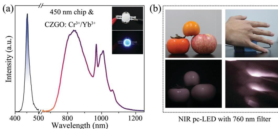
Fig. 8 (a) The output spectrum of fabricated NIR pc-LED packaged by combining a 450 nm chip with CZGO: Cr<sup>3+</sup>/Yb<sup>3+</sup>. The inset shows the fabricated LED devices. (b) Photographs of various fruit and a hand under a white LED and NIR pc-LED with a 760 nm filter.
