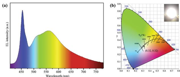
**Fig. 8** (a) EL emissive spectra of a WLED fabricated by the green  $\text{Lu}_3\text{Al}_5\text{O}_{12}:\text{Ce}^{3+}$  phosphors and yellow-emissive AIS/ZnS core/shell QDs, and (b) the corresponding CIE color coordinates of WLED and a photograph of the device operated at 200 mA (inset). Copied with permission.<sup>85</sup>
