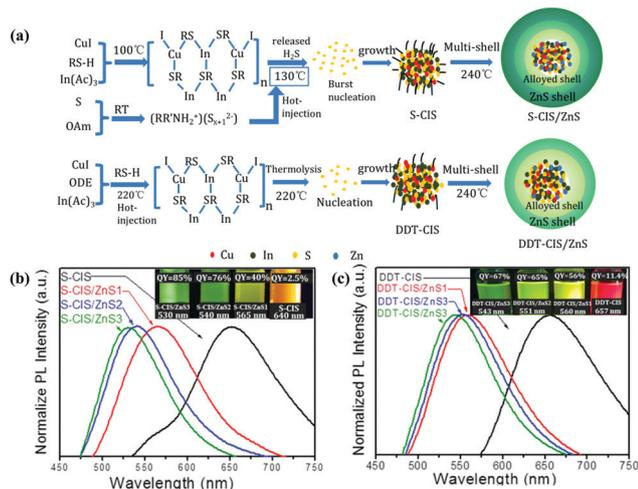
**Fig. 3** (a) Schematic illustration of the formation process of CIS/ZnS QDs with S-OAm (S-CIS/ZnS) and 1-dodecanethiol (DDT-CIS/ZnS) as the sulfur source. Normalized PL emission spectra and photographs of the samples under 365 nm UV illumination (inset) of (b) S-CIS/ZnS and (c) DDT-CIS/ZnS QDs. Reproduced with permission.<sup>39</sup> Copyright 2020 Published by Elsevier B.V.
