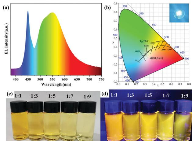
**Fig. 5** (a) Electroluminescent (EL) spectrum, (b) the corresponding Commission Internationale de l'Eclairage (CIE) color coordinates and a photograph (inset) of the WLED operating at 50 mA. Photographs of AIZS QDs with different Ag/In ratios under (c) daylight and (d) UV light. Copied with permission.<sup>42</sup> Copyright 2020 Elsevier B.V. All rights reserved.
