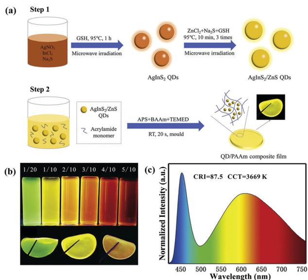
**Fig. 9** (a) Synthetic illustration for the preparation of AIS/ZnS QDs and QD/PAAm composite film for WLEDs. (b) Digital photographs of AIS/ZnS QDs synthesized at different molar ratios of Ag/In (above) and QD/PAAm composite films of green, yellow, and red (below) under UV irradiation. (c) Emission spectrum of the LED based on green and red QD/PAAm films at a drive current of 20 mA. Reproduced with permission.<sup>85</sup> Copyright 2020 Elsevier B.V. All rights reserved.
