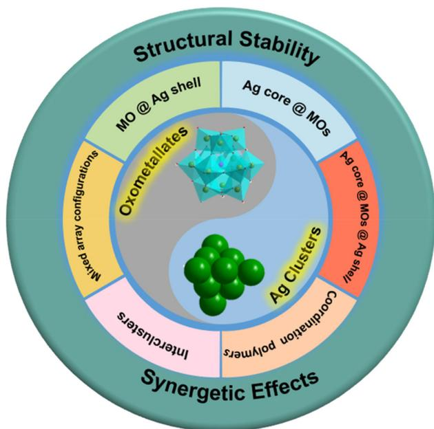
**Scheme 1** The schematic diagram of the assembly modes which are classified into six types, including MO @ Ag shells, Ag core @ MOs, Ag core @ MOs @ Ag shells, coordination polymers, intercluster compounds and mixed array configurations.
