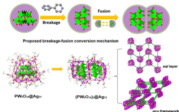
Fig. 6 Molecular structures of  $\text{PW}_9\text{O}_{34}@Ag_{51}$  and  $(\text{PW}_9\text{O}_{34})_2@Ag_{72}$  (left), and the two simplified networks with  $(\text{PW}_9\text{O}_{34})_2@Ag_{72}$  as the node (yellow balls) and bipy as the linker (right). Reproduced with permission from ref. 33. Copyright 2022, Nature Publishing Group.
