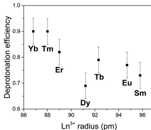
**Fig. 6** Deprotonation efficiency of  $\{\text{Ln}_4\text{Nb}_{28}\}$  clusters versus the ionic radii of  $\text{Ln}^{\text{III}}$  centers. The deprotonation efficiency, which is calculated by the ratio of the number of protons released per entire POM molecule over the molar ratio of KOH/cluster, indicates the number of protons released per entire POM molecule with the introduction of 1 equiv. of KOH.
