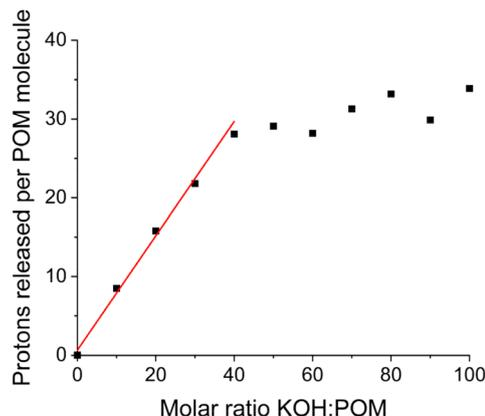
Fig. 4 The number of protons released per molecular cluster (including the protons contributed by the hydrolysis of ammonium ions) versus the molar ratio of KOH introduced to  $\{\text{Sm}_4\text{Nb}_{28}\}$  clusters.
