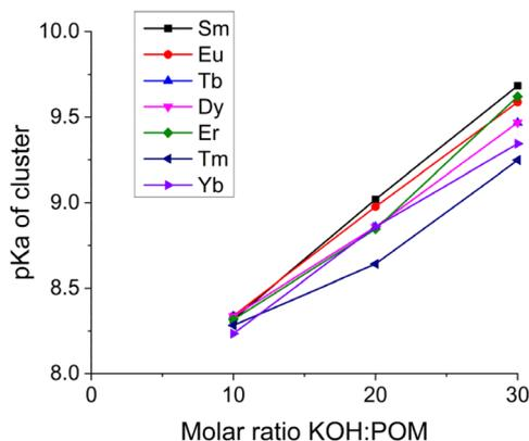
Fig. 7 The  $pK_a$  values of the  $\{Ln_4Nb_{28}\}$  clusters during the deprotonation process.
