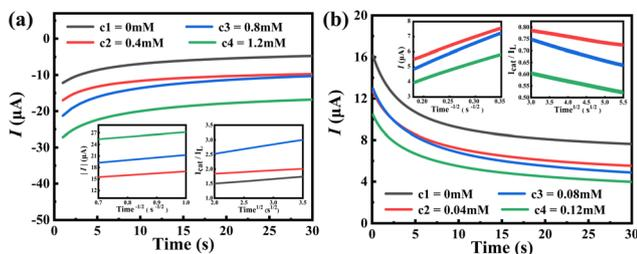
**Fig. 8** (a) Chronoamperometry on hybrid **1** after the successive addition of different concentrations of Cr(vi) in  $0.5 \text{ M H}_2\text{SO}_4$ ; (b) Chronoamperometry on hybrid **1** after the addition of different concentrations of TC in  $0.5 \text{ M H}_2\text{SO}_4$ . Insets left: plots of  $I_{\text{cat}}/I_L$  versus  $t^{1/2}$ ; right:  $I$  versus  $t^{-1/2}$ .
