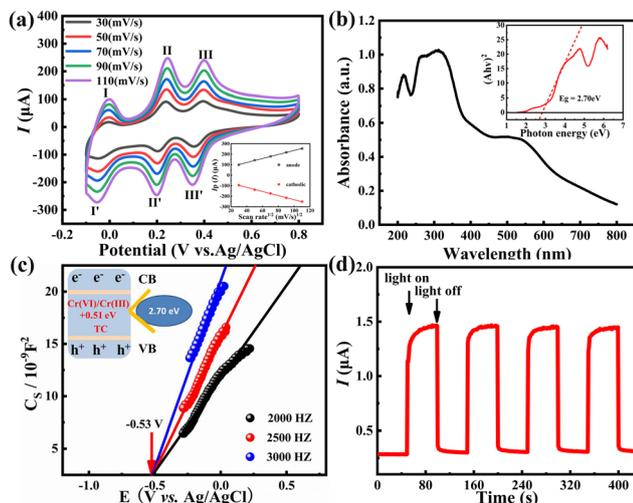
**Fig. 3** (a) CV curves of hybrid **1** at different scan rates; (b) UV-vis diffuse reflection spectrum of **1**, inset: the corresponding plot of  $(ah\nu)^2$  vs.  $h\nu$ ; (c) Mott–Schottky plots of **1** in 0.2 M  $\text{Na}_2\text{SO}_4$  solution at pH = 6.80, inset: energy diagram of the HOMO and LUMO levels of **1**; (d) Transient photocurrent response of hybrid **1** within four cycles of light on/off.
