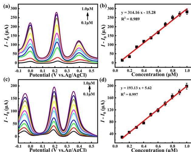
**Fig. 7** (a) DPV curves of hybrid **1** in acidified lake water with continuous addition of TC; (b) The linear dependence curve of **1**; (c) DPV curves of hybrid **1** in acidified milk with continuous addition of TC; (d) The linear dependence curve of **1**.
