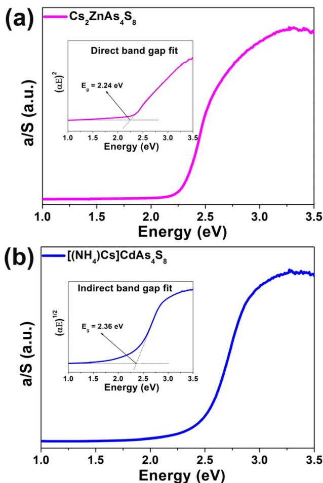
Fig. 2 UV-vis-NIR diffuse reflectance spectra of (a)  $\text{Cs}_2\text{ZnAs}_4\text{S}_8$  and (b)  $[(\text{NH}_4)\text{Cs}]\text{CdAs}_4\text{S}_8$  (inset: direct or indirect band gap fit based on the DFT results).
