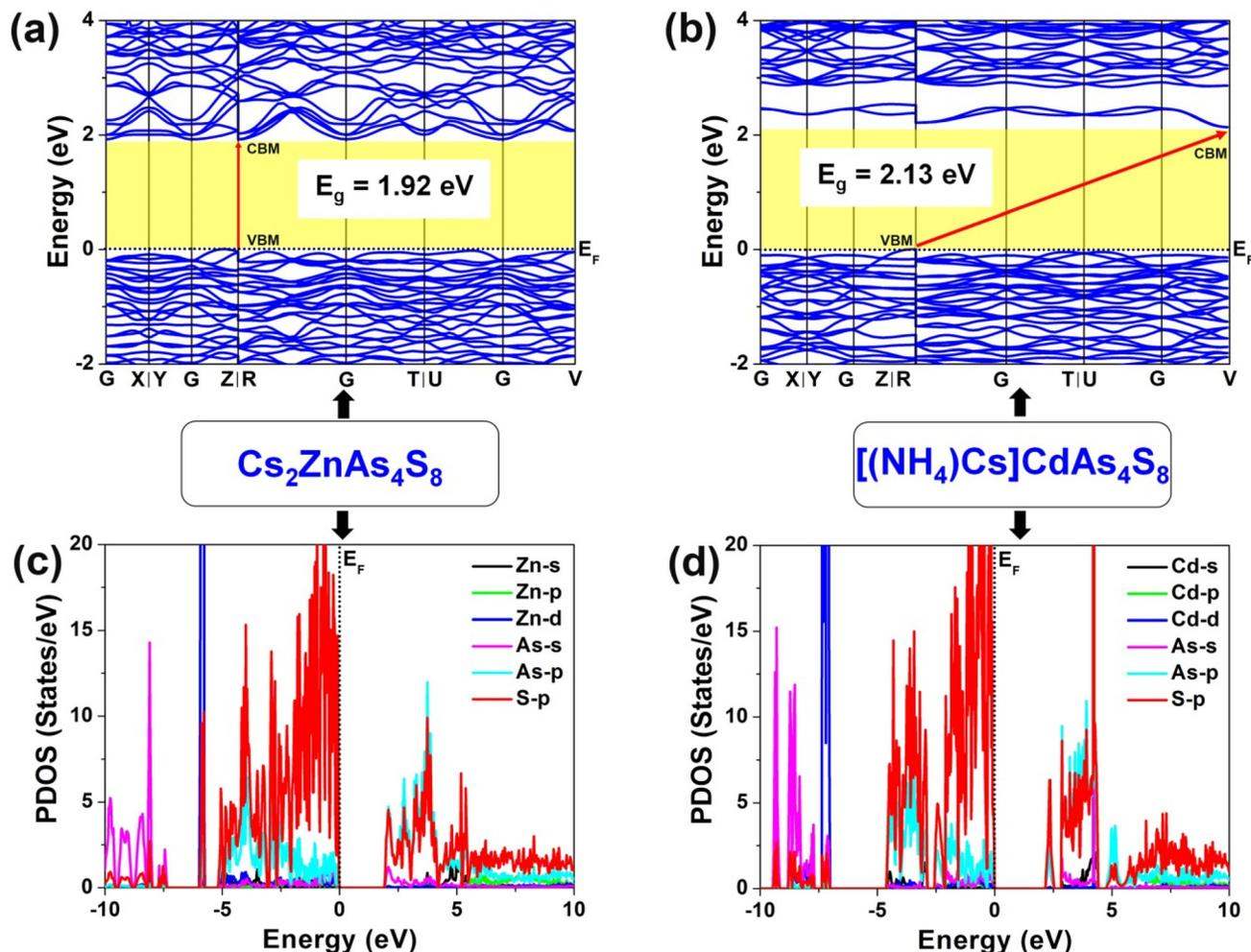
Fig. 4 Theoretical calculated results of  $\text{Cs}_2\text{ZnAs}_4\text{S}_8$  and  $[(\text{NH}_4)\text{Cs}]\text{CdAs}_4\text{S}_8$ : (a, b) electronic band structures; (c, d) PDOSs (states with fewer contributions are omitted for a better view). The Fermi level  $E_F$  is set at 0.0 eV.
