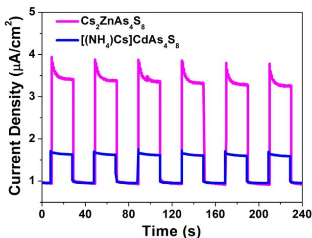
Fig. 3 Photocurrent response curves of  $\text{Cs}_2\text{ZnAs}_4\text{S}_8$  and  $[(\text{NH}_4)\text{Cs}]\text{CdAs}_4\text{S}_8$ .
