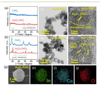
Fig. 1 (a) XRD patterns of  $CeO_x$  and  $In_2O_3-CeO_{x_r}$  (b) XRD patterns of  $CeO_2$  and  $In_2O_3-CeO_2$ , (c and d) HR-TEM image of  $In_2O_3-CeO_x$  and (e and f) HR-TEM image of In<sub>2</sub>O<sub>3</sub>-CeO<sub>2</sub>. (g-j) The corresponding EDX elemental mapping of In2O3CeOx.
