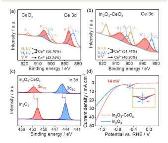
Fig. 2 Ce 3d XPS spectra of (a) CeO<sub>x</sub> and (b) In<sub>2</sub>O<sub>3</sub>-CeO<sub>x</sub>; (c) In 3d XPS spectra of  $ln_2O_3$ -CeO<sub>x</sub> and  $ln_2O_3$ ; and (d) LSVs of  $ln_2O_3$  and  $ln_2O_3$ - $CeO_x$  in  $CO_2$ -saturated 0.5 M KHCO<sub>3</sub> at a scan rate of 50 mV s<sup>-1</sup>.
