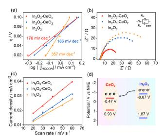
Fig. 4 Advantages of In<sub>2</sub>O<sub>3</sub>-CeO<sub>x</sub> for CO<sub>2</sub> reduction. (a) Tafel plots, (b) Nyquist plots (inset: equivalent circuit), (c) linear fitting of double-layer capacitive currents versus scan rates to estimate the ECSA of In<sub>2</sub>O<sub>3</sub>-CeO<sub>x</sub>, In<sub>2</sub>O<sub>3</sub>-CeO<sub>2</sub> and In<sub>2</sub>O<sub>3</sub>, and (d) schematic illustration of the charge transfer in In<sub>2</sub>O<sub>2</sub>-CeO<sub>4</sub>
