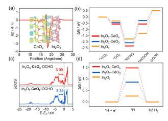
Fig. 5 DFT calculations. (a) Charge density difference and charge displacement curves of In<sub>2</sub>O<sub>3</sub>-CeO<sub>x</sub>; purple, yellow, and red spheres represent In, Ce, and O atoms, respectively. (b) Gibbs free-energy diagrams of CO2-to-formate. (c) In-5p p-DOS of In2O3-CeOx and In2O3-CeO2 after adsorbing \*OCHO. (d) Gibbs free-energy diagrams of the HER.
