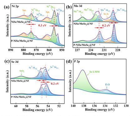
Fig. 3 XPS spectra of (a) Ni 2p, (b) Mo 3d, (c) Se 3d in NiSe/MoSe<sub>2</sub>@NF and P-NiSe/MoSe<sub>2</sub>@NF. (d) XPS spectrum of P 2p in P-NiSe/MoSe<sub>2</sub>@NF.
