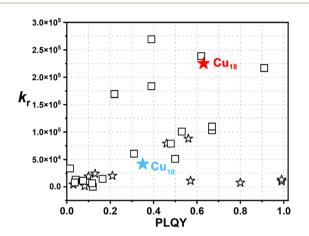
Fig. 1 Summary of calculated radiative decay rate  $(k_r = \Phi/\tau)$  versus PLQY ( $\Phi$ ) of all reported atomically precise CuNCs, including protected S<sup>-</sup>, P<sup>-</sup> and I ligands (squares) and C≡C<sup>-</sup> (pentagons) (see Table S5† for details)
