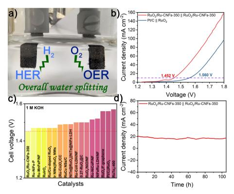
Fig. 5 Overall water splitting measurements in 1 M KOH. (a) Digital graph of the  $RuO_2/Ru$ -CNFs-350| $RuO_2/Ru$ -CNFs-350 electrolyzer. (b) Polarization curves of the  $RuO_2/Ru$ -CNFs-350| $RuO_2/Ru$ -CNFs-350
