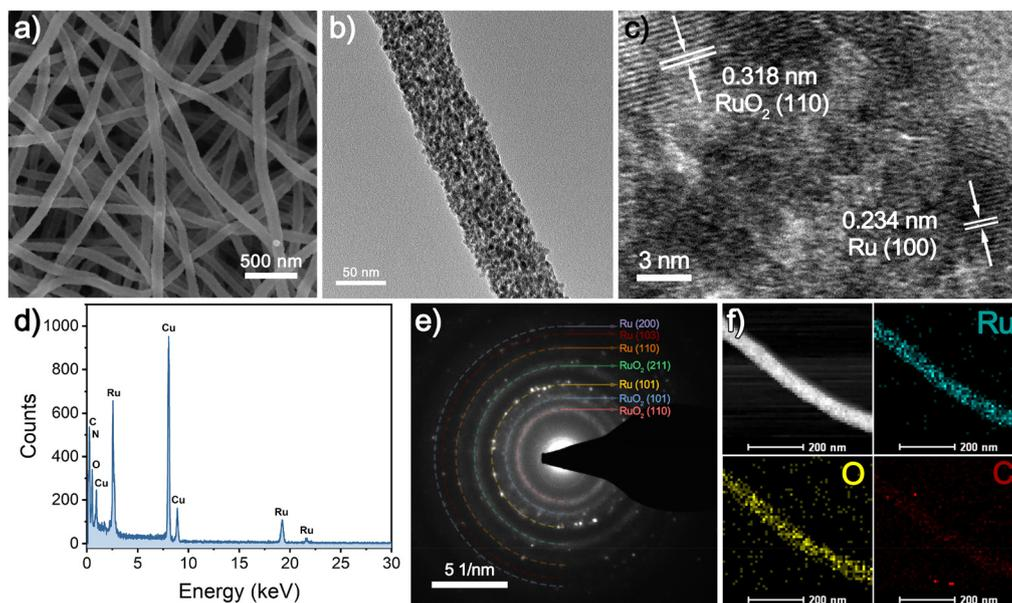
**Fig. 1** (a) SEM image, (b) TEM image, (c) HRTEM image, (d) EDX spectrum, (e) SAED pattern, (f) HAADF-STEM micrograph and EDX mappings of synthesized RuO<sub>2</sub>/Ru-CNFs-350.
