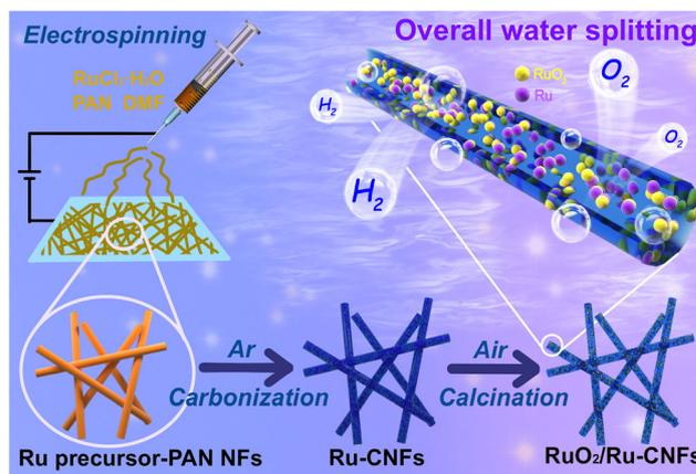
Scheme 1 Schematic diagram of the fabrication of  $\text{RuO}_2/\text{Ru-CNFs}$ .
