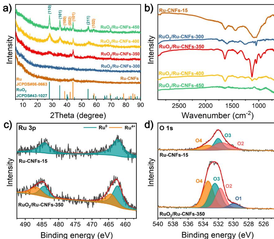
**Fig. 2** (a) XRD patterns and (b) FT-IR spectra of Ru-CNFs-15 and different RuO<sub>2</sub>/Ru-CNF catalysts. Narrow-scan XPS spectra of (c) Ru 3p and (d) O 1s of Ru-CNFs-15 and RuO<sub>2</sub>/Ru-CNFs-350.
