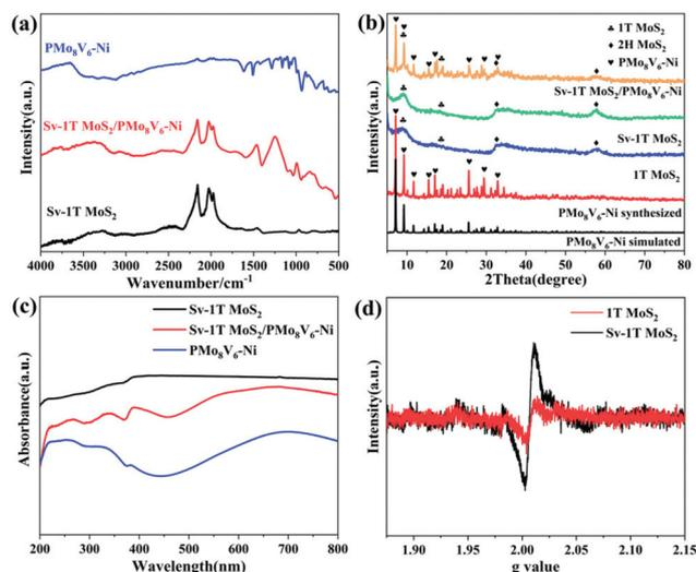
**Fig. 3** (a) FT-IR spectra, (b) XRD patterns, and (c) UV-vis diffuse reflectance spectra of Sv-1T MoS<sub>2</sub>, PMo<sub>8</sub>V<sub>6</sub>-Ni, and Sv-1T MoS<sub>2</sub>/PMo<sub>8</sub>V<sub>6</sub>-Ni composite-materials, and (d) EPR spectra of 1T MoS<sub>2</sub> and Sv-1T MoS<sub>2</sub>.
