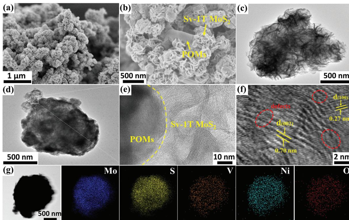
**Fig. 2** (a) SEM and (c) TEM images of Sv-1T MoS<sub>2</sub>; (b) SEM, (d) TEM, and (e), (f) HRTEM of the Sv-1T MoS<sub>2</sub>/PMo<sub>8</sub>V<sub>6</sub>-Ni composite-material; (g) EDX mapping of Mo, S, V, Ni, and O in the Sv-1T MoS<sub>2</sub>/PMo<sub>8</sub>V<sub>6</sub>-Ni composite-material.
