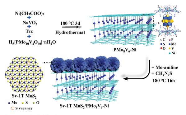
Scheme 1 Illustration of the Sv-1T MoS<sub>2</sub>/PMo<sub>8</sub>V<sub>6</sub>-Ni preparation process.
