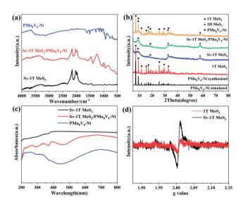
Fig. 3 (a) FT-IR spectra, (b) XRD patterns, and (c) UV-vis diffuse reflectance spectra of Sv-1T MoS<sub>2</sub>, PMo<sub>8</sub>V<sub>6</sub>-Ni, and Sv-1T MoS<sub>2</sub>/PMo<sub>8</sub>V<sub>6</sub>-Ni composite-materials, and (d) EPR spectra of 1T  $MoS_2$  and Sv-1T  $MoS_2$ .
