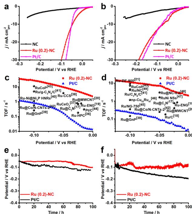
**Fig. 2** Electrocatalytic HER performance of Ru (0.2)-NC and other control catalysts. (a and b) LSV curves. Scan rate: 5 mV s<sup>-1</sup>. (c and d) Comparison of the TOF values with other start-of-the-art Ru-based HER catalysts. (e and f) Long-term catalytic stability test at –10 mA cm<sup>-2</sup>. Data were acquired in (a, c and e) 0.5 M H<sub>2</sub>SO<sub>4</sub> and (b, d and f) 1.0 M KOH, respectively.
