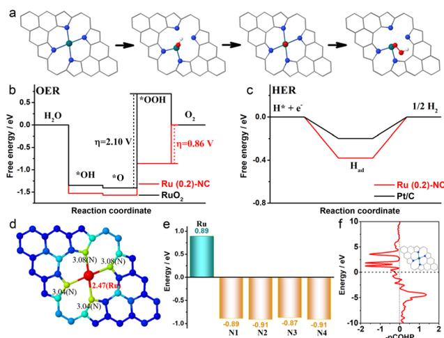
**Fig. 4** (a) Adsorption configurations of the intermediates during the OER process on pyrrole-type Ru (0.2)-NC (the balls in cyan, blue, red and white represent Ru, N, O and H atoms, respectively). Gibbs free energy diagrams for (b) the four steps of OER and (c) the two steps of HER on pyrrole-type Ru (0.2)-NC. The dotted lines in panel (b) denote the RDS. (d) The band-order, (e) Bader charge and (f) COHP analyses of pyrrole-type Ru (0.2)-NC.
