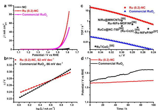
**Fig. 3** Electrocatalytic OER performance of Ru (0.2)-NC and other control catalysts. (a) LSV curves. Scan rate: 5  $\text{mV s}^{-1}$ . (b) Tafel slopes. (c) Comparison of the TOF values with other start-of-the-art OER catalysts. (d) Long-term catalytic stability test at 10  $\text{mA cm}^{-2}$  in 1.0 M KOH.
