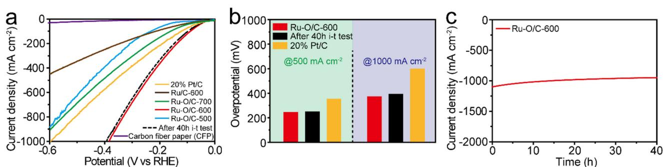
**Fig. 7** HER performance under large-current conditions. (a) LSV curves of Ru–O/C-600, 20% Pt/C and carbon fiber paper (CFP) in 1 M KOH; the dashed lines in (a) refer to the LSV curves of Ru–O/C-600 CFP after the 40 h *i*–*t* test. (b) Comparison of the overpotentials at the current densities of 500 and 1000 mA cm<sup>−2</sup> for Ru–O/C-600 and 20% Pt/C, both in 1 M KOH. (c) Long-term chronoamperometric testing of Ru–O/C-600 in 1 M KOH at a current density of 1000 mA cm<sup>−2</sup>.
