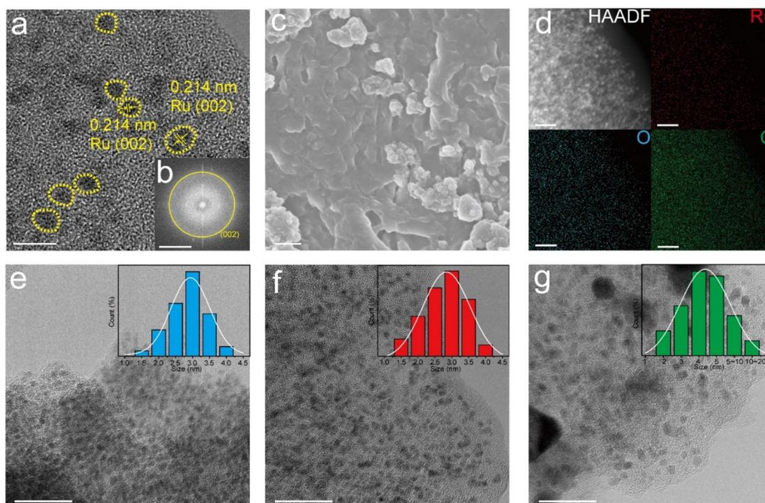
**Fig. 3** (a) HRTEM, (b) SAED, (c) SEM and (d) HAADF-TEM images and the corresponding elemental mapping of Ru, C and O for Ru-O/C-600. HRTEM images of (e) Ru-O/C-500, (f) Ru-O/C-600 and (g) Ru-O/C-700. Scale bar: (a–g) 5 nm, 21/nm, 1  $\mu$ m, 20 nm, 20 nm, 20 nm, and 20 nm, respectively.
