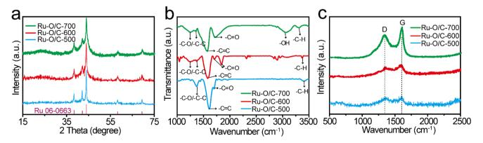
Fig. 2 Structure characterization of Ru-O/C-600, Ru-O/C-700 and Ru-O/C-500. (a) XRD patterns, (b) FT-IR spectra and (c) Raman spectra of Ru-O/C-600 (red), Ru-O/C-700 (green) and Ru-O/C-500 (blue).
