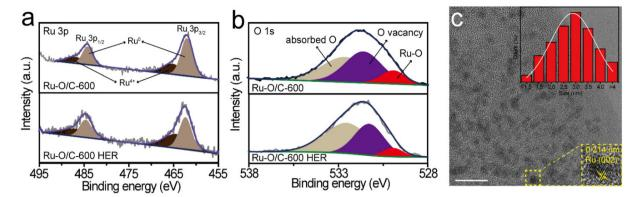
Fig. 6 The Ru-O/C-600 results after long-time stability testing. High-resolution XPS spectra of (a) Ru 3p and (b) O 1s. (c) TEM image. Scale bar:
