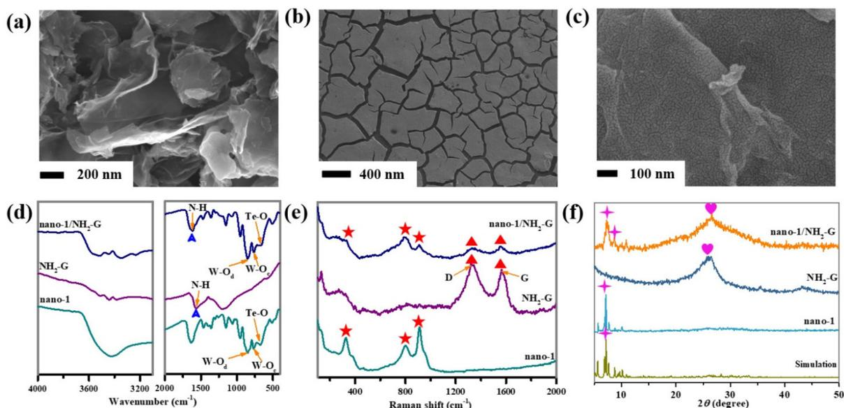
**Fig. 4** (a–c) SEM images of **NH<sub>2</sub>-G**, **nano-1** and **nano-1/NH<sub>2</sub>-G**. (d) IR spectra, (e) Raman spectra and (f) PXRD patterns of simulation of **1**, **nano-1**, **NH<sub>2</sub>-G**, and **nano-1/NH<sub>2</sub>-G**.
