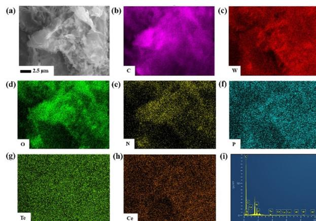
**Fig. 5** (a) SEM image of nano-1/NH<sub>2</sub>-G at the 2.5 μm scale. (b–h) SEM-EDS C, W, O, N, P, Te and Ce elemental mapping images of nano-1/NH<sub>2</sub>-G on a silicon substrate. (i) EDS of nano-1/NH<sub>2</sub>-G.
