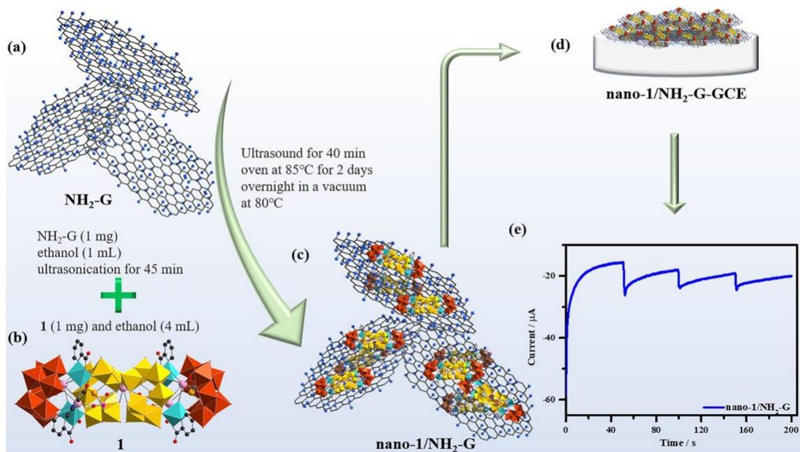
**Scheme 1** Schematic preparation process of nano-1/NH<sub>2</sub>-G-GCE. (a) Schematic structure of NH<sub>2</sub>-G. (b) Crystal structure of 1. (c) Schematic structure of nano-1/NH<sub>2</sub>-G. (d) The nano-1/NH<sub>2</sub>-G-GCE. (e) Schematic detection curve.
