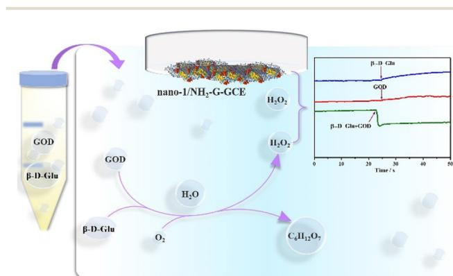
**Fig. 8** Schematic enzyme electrochemical glucose sensing system and ARCs of the **nano-1/NH<sub>2</sub>-G-GCE** sensor with the addition of β-D-Glu, GOD and β-D-Glu + GOD in 0.1 M PBS (pH = 6.5) at –0.20 V.
