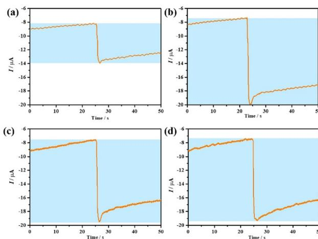
**Fig. 9** (a–d) ARCs of **nano-1/NH<sub>2</sub>-G-GCE** towards a β-D-Glu + GOD solution at heating times of 0, 30, 60 and 90 min, respectively. The tests were carried out in 0.1 M PBS (pH = 6.5) at –0.20 V.
