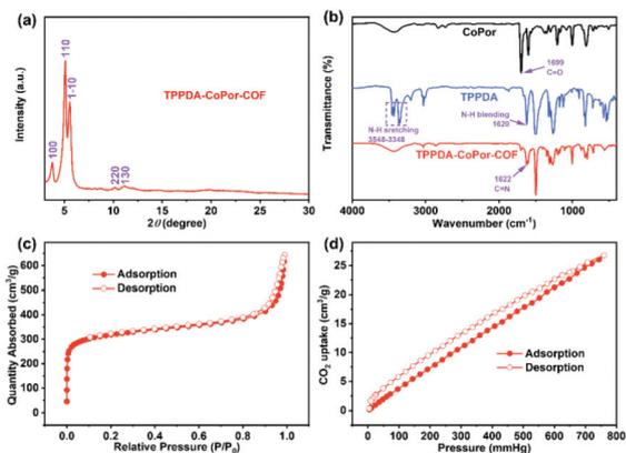
Fig. 2 (a) Experimental PXRD patterns, (b) FT-IR spectra, (c) N<sub>2</sub> sorption isotherm at 77 K and (d) CO<sub>2</sub> sorption isotherm at 298 K for TPPDA-CoPor-COF.
