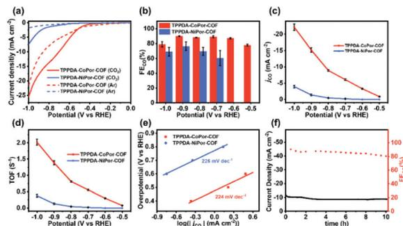
Fig. 5 (a) LSV curves, (b) FE<sub>CO</sub>, (c) *j*<sub>CO</sub>, (d) TOF and (e) Tafel plots of TPPDA-MPor-COFs. (f) Lasting stability test for TPPDA-CoPor-COF at –0.8 V.
