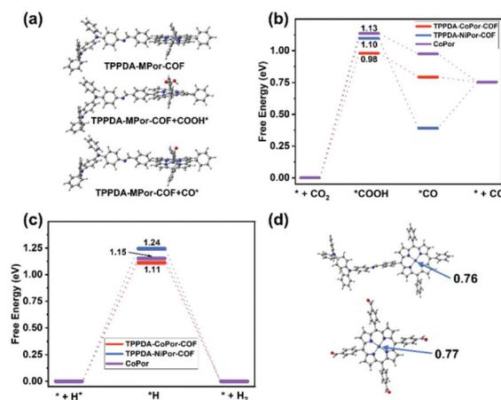
**Fig. 7** (a) The proposed mechanism of the electrocatalytic CO<sub>2</sub>RR for TPPDA-MPor-COFs. (b) The calculated energy diagrams of CO<sub>2</sub> reduction to CO and (c) the calculated energy diagrams of the HER for TPPDA-MPor-COFs and CoPor. (d) The Mulliken charge of the Co site in TPPDA-CoPor-COF and CoPor.
