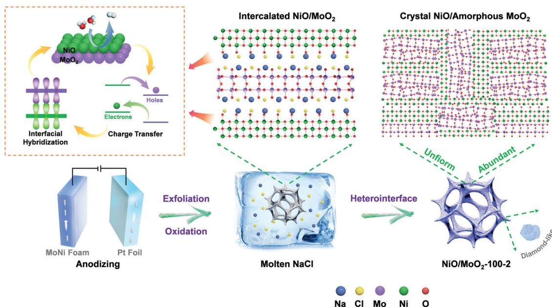
**Scheme 1** Illustration of the fabrication process of the NiO/MoO<sub>2</sub>-100-2 sample.
