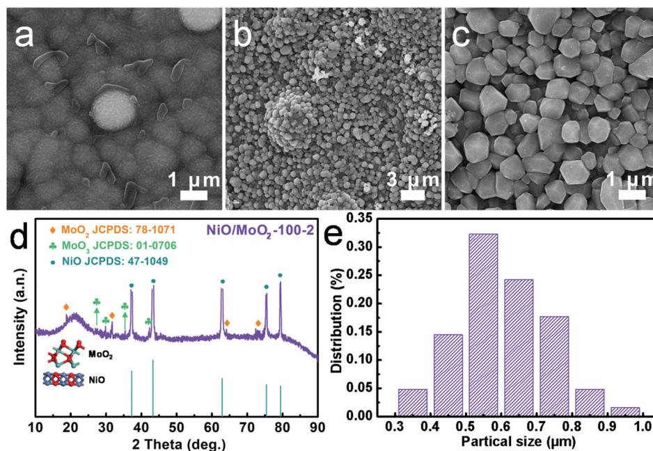
**Fig. 1** Structure characterization of NiO/MoO<sub>2</sub>-100 and NiO/MoO<sub>2</sub>-100-2. SEM images of (a) NiO/MoO<sub>2</sub>-100 and (b and c) NiO/MoO<sub>2</sub>-100-2. (d) XRD pattern and (e) particle distribution of NiO/MoO<sub>2</sub>-100-2.
