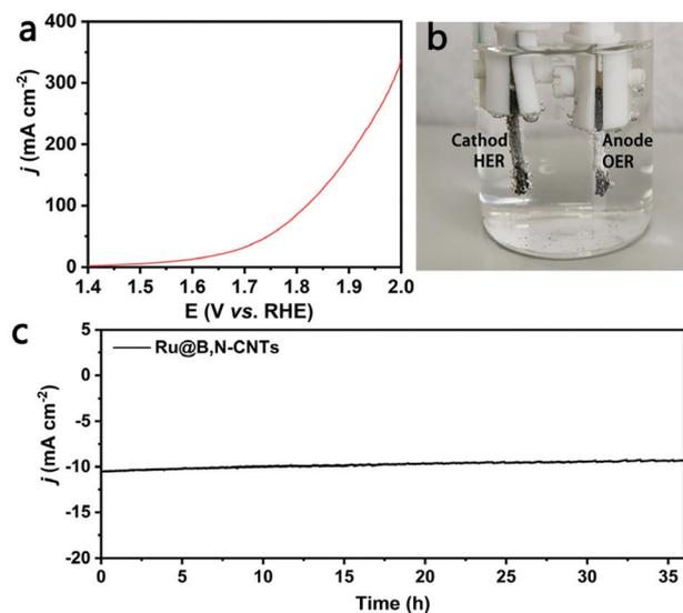
**Fig. 6** (a) The LSV curve for the assembled electrolyzer in 1 M KOH employing Ru@B,N-CNT electrocatalysts as both anode and cathode. (b) A photograph of the assembled electrolyzer using Ru@B,N-CNTs as both cathode and anode. (c) The chronoamperometric  $i-t$  curve measured at an applied potential of 1.57 V for the electrolyzer assembled with Ru@B,N-CNT electrocatalysts for 36 h.
