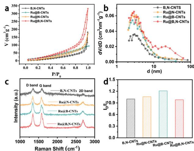
Fig. 3 (a) The N<sub>2</sub> sorption isotherms, (b) the corresponding pore size distributions, (c) the Raman spectra, and (d) the corresponding  $I_D/I_G$  ratios, of the B,N-CNTs, Ru@B,-CNTs, Ru@N-CNTs and Ru@B,N-CNTs.
