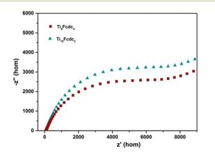
Fig. 6 Electrochemical impedance spectroscopy of clusters Ti<sub>8</sub>Fcdc<sub>4</sub> and Ti<sub>10</sub>Fcdc<sub>2</sub>
