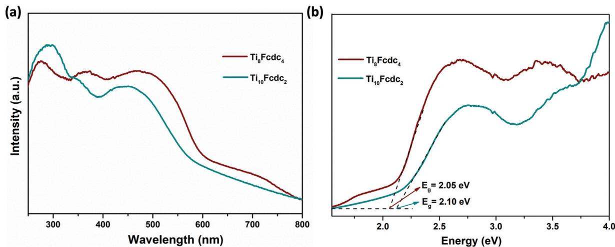
Fig. 3 (a) The solid-state UV-vis spectra of clusters  $\text{Ti}_8\text{Fcdc}_4$  and  $\text{Ti}_{10}\text{Fcdc}_2$ . (b) Kubelka-Munk transformation of diffuse reflectance data of clusters  $\text{Ti}_8\text{Fcdc}_4$  and  $\text{Ti}_{10}\text{Fcdc}_2$ .
