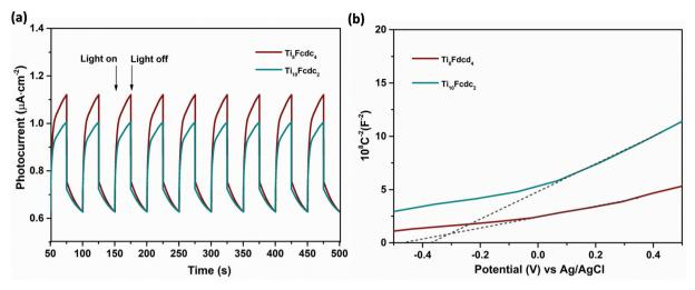
Fig. 5 (a) The photocurrent responses of clusters Ti<sub>8</sub>Fcdc<sub>4</sub> and Ti<sub>10</sub>Fcdc<sub>2</sub>. (b) The Mott–Schottky plots of clusters Ti<sub>8</sub>Fcdc<sub>4</sub> and Ti<sub>10</sub>Fcdc<sub>2</sub>.
