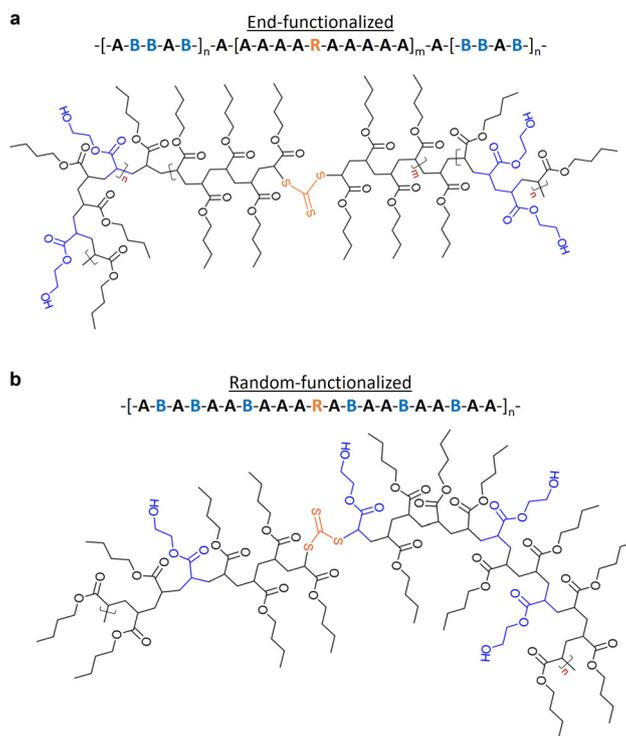
**Fig. 1** Representation of prepolymer structures with the HEA (B) located on the (a) end and (b) randomly distributed on the BA (A) chain. Both prepolymers are formed using a 4 : 1 (w/w) BA/HEA ratio and a RAFT agent (R).
