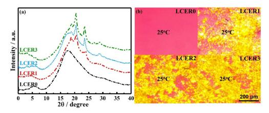
Fig. 5 (a) WAXD curves and (b) POM images of LCERs at 25 °C.
