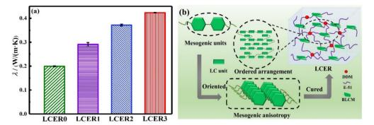
Fig. 4 (a) Thermal conductivities (λ) of LCERs; (b) schematic diagram of a mesomorphic phase arrangement within the cured epoxy network.
