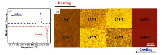
Fig. 2 (a) DSC curves and (b) POM images during the heating and cooling processes of BLCM.
