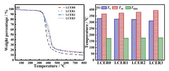
Fig. 6 (a) TGA curves and (b) characteristic thermal data of LCERs
