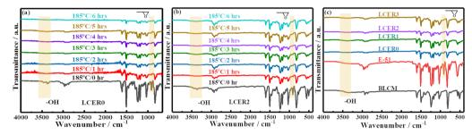
Fig. 3 FT-IR spectra of (a) LCER0 and (b) LCER2 at different time during the curing process; (c) FT-IR spectra of cured LCERs, E-51, and BLCM.
