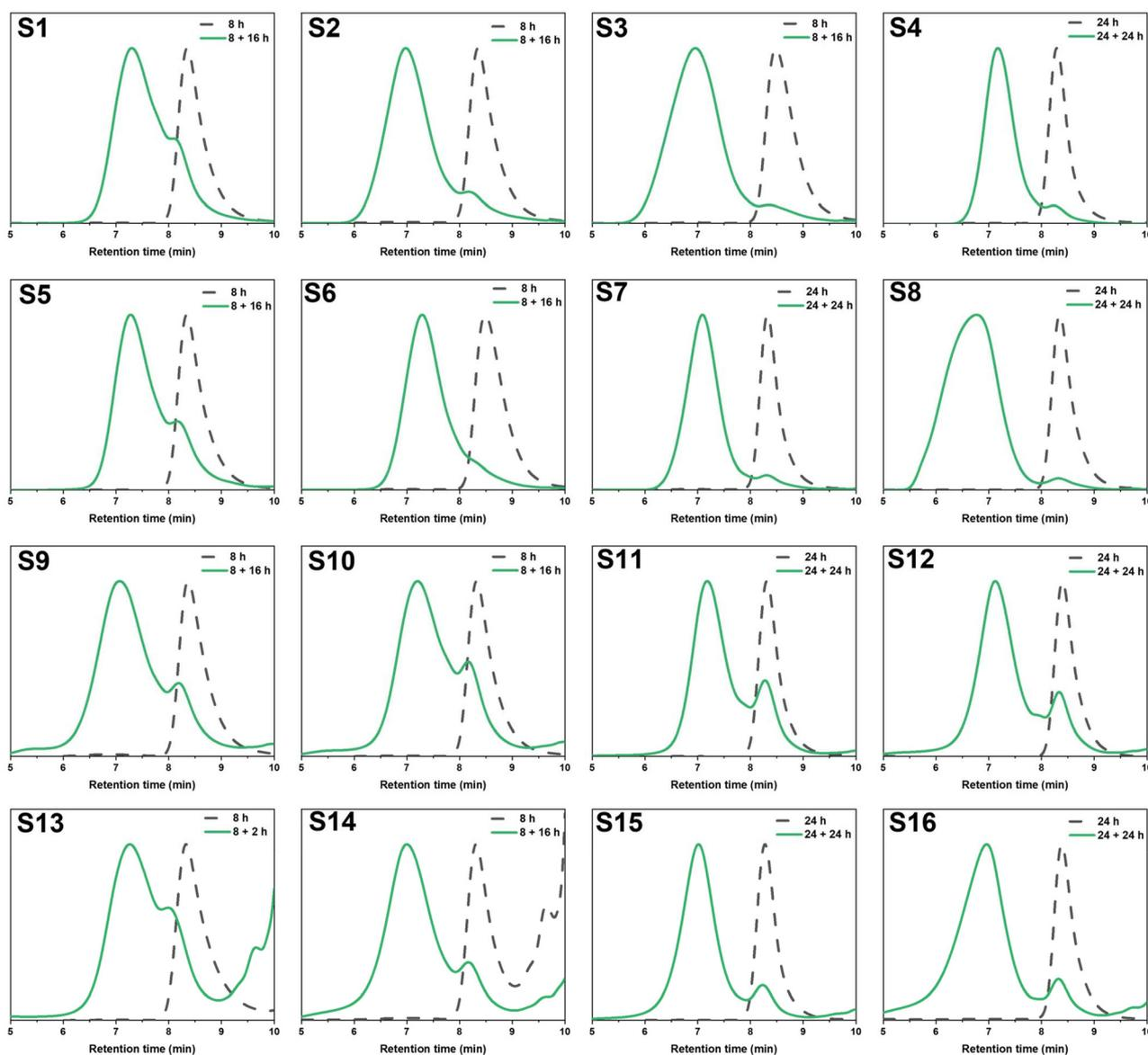
**Fig. 3** GPC traces of branched core-crosslinked polymers **S1**–**S16** before (dashed) and after (solid) the addition of the crosslinker and their subsequent shifts to higher molecular weight. For **S13**, a sample is shown after 8 + 2 h due to gelation after the full reaction time.
