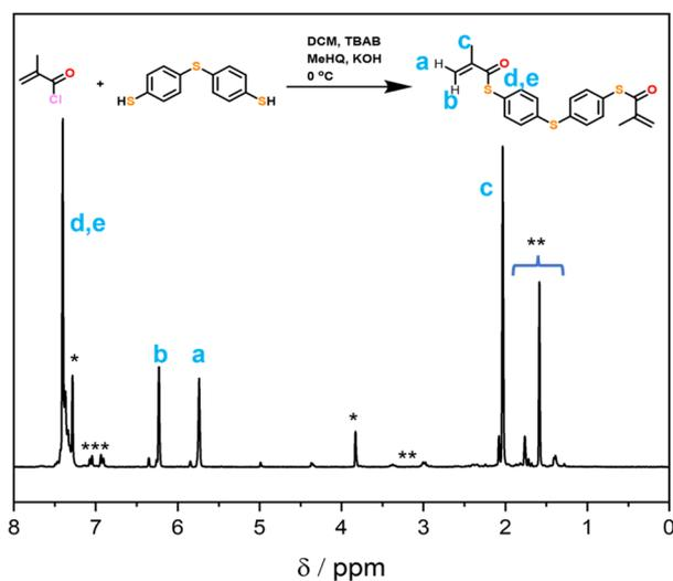
**Fig. 2**  $^1\text{H}$  NMR ( $\text{CDCl}_3$ ) of the crude bifunctional thiomethacrylate crosslinker. Impurity peaks are identified as residual inhibitor *p*-methoxyphenol (MeHQ, \*), tetrabutyl ammonium bromide (TBAB, \*\*) and toluene (\*\*\*).
