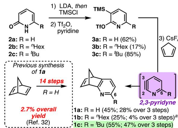
**Fig. 2** Synthesis of pyridinonorbornenes **1a–c** *via* 2,3-pyridynes. Reagents and conditions: (1) LDA (2.2 equiv.), THF, 0 °C, 1 h, then TMSCl (1.2 equiv.), 0 °C, 15 min, then rt, 12 h. (2) Tf<sub>2</sub>O (1.1 equiv.), pyridine, 0 °C, 20 min, then rt, 12 h. (3) CsF (5.0 equiv.), C<sub>5</sub>H<sub>6</sub> (5.0 equiv.), MeCN, 30 °C, 3 h. <sup>a</sup>4 : 1 MeCN : DCM.
