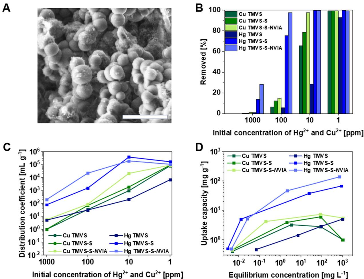
Fig. 2 (A) SEM image of TMVS-S-NVIA particles. Scalebar is 5  $\mu\text{m}$ . (B) Removed copper ions (green) and mercury ions (blue) from aqueous solution by TMVS-S and TMVS-S-NVIA particles in %. Calculated distribution coefficients (C) and uptake capacities (D) of TMVS-S particles and TMVS-S-NVIA particles, respectively. Uptake capacities plotted against initial ion concentration can be found in the ESI.†
