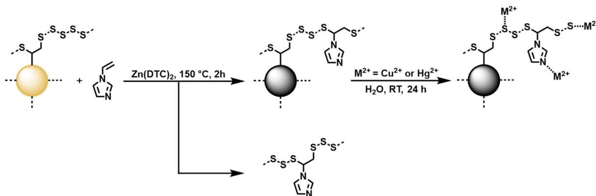
**Scheme 2** Reaction equation of the dynamic covalent polymerization of inverse vulcanized TMVS-S particles with *N*-vinylimidazole to create TMVS-S-NVIA particles and their adsorption of  $\text{Hg}^{2+}$  and  $\text{Cu}^{2+}$  ions. Sulfur chains are abbreviated with dashed lines.
