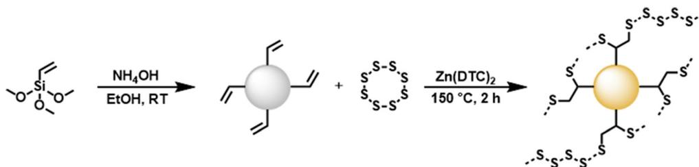
**Scheme 1** Reaction equation of the inverse vulcanization of vinylated TMVS particles made by a modified Stöber method. Sulfur chains are abbreviated by dotted lines.
