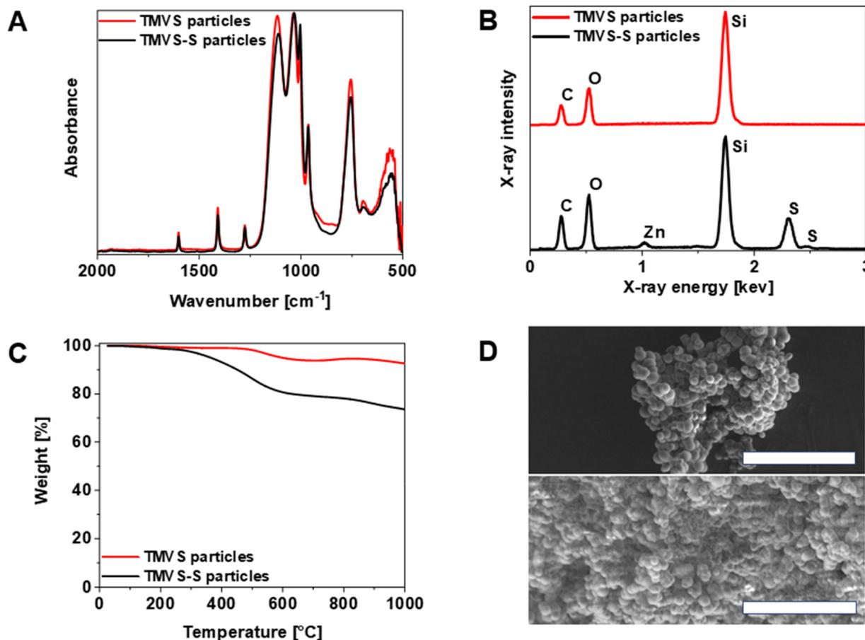
**Fig. 1** Normalized ATR FT-IR (A) and normalized EDX (B) spectra of TMVS and TMVS-S particles, respectively. (C) Thermograms of TMVS and TMVS-S particles up to 1000 °C. (D) SEM image of TMVS particles (upper image) and inverse vulcanized TMVS-S particles (lower image). Scalebar is 20  $\mu\text{m}$ .
